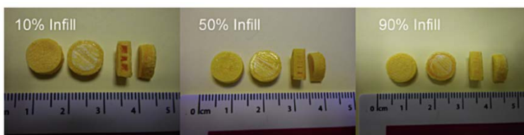
Figure 21 Images of 3D Printed Tablets as a Function of Infill Percentage (2)
