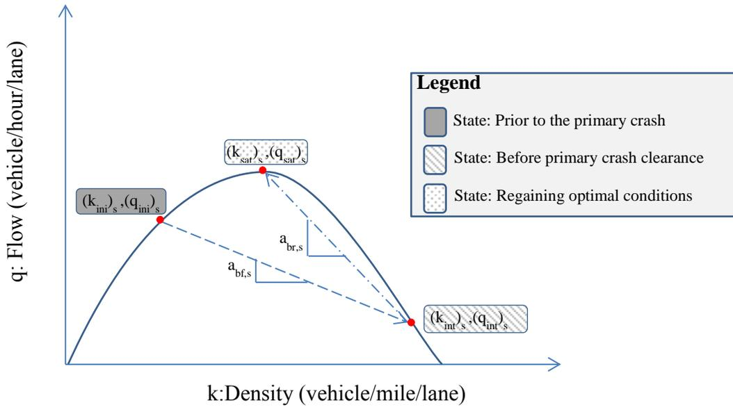
(a) Determining shockwave speed in same direction using traffic flow characteristics.
