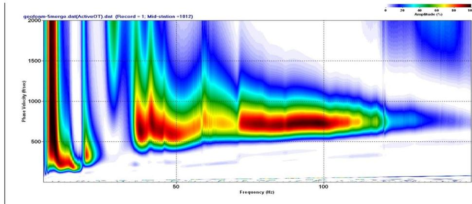
Figure 8. Dispersion curve from Surfseis for station # 5.75.
