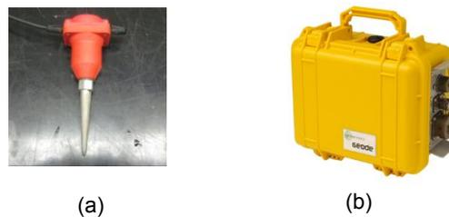
Figure 2. (a) 4.5 Hz geophone, (b) Geode
