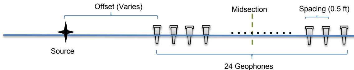
Figure 3. Source-receiver configuration for active MASW test
