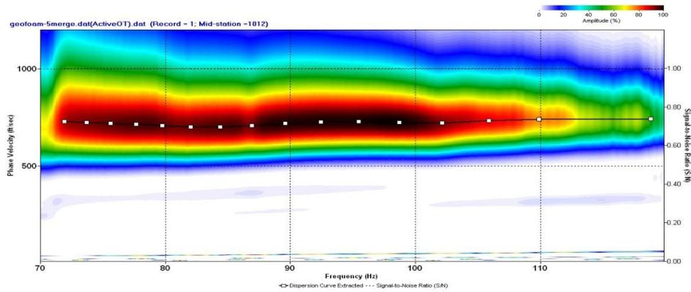
Figure 9. Extracted dispersion curve from Surfseis for station # 5.75.
