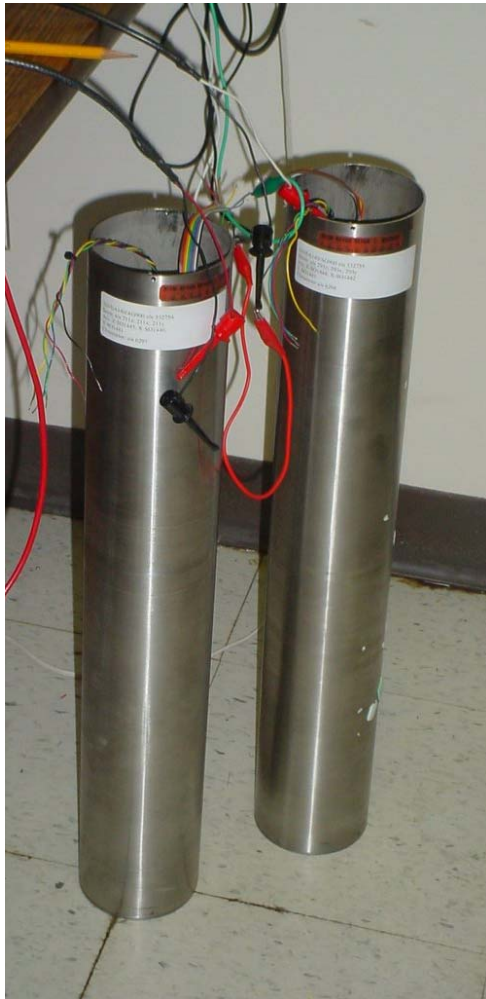
Figure 6. Custom shallow borehole packages incorporating triaxial broadband and accelerometer sensor components.
