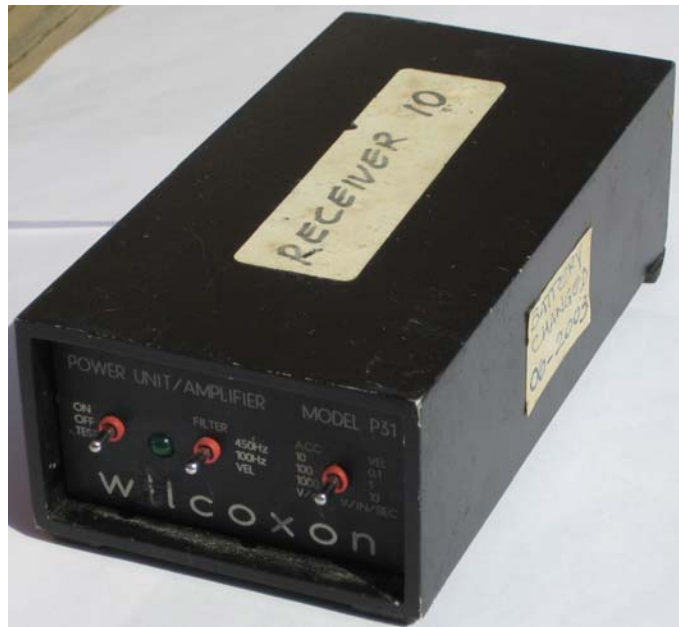
Figure 4.7 Wilcox P31 Power Unit/Amplifier with optional gain and filter settings.
