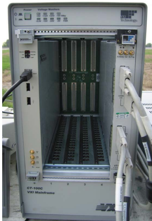
Figure 4.8 CT-100C portable VXIbus mainframe with slotted VT1432A 16-channel 24-bit digitizer.
