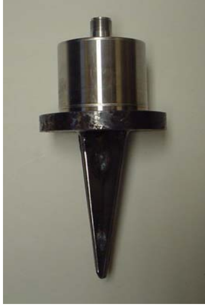
Figure 4.6 Wilcox 731A Seismic Accelerometer.
