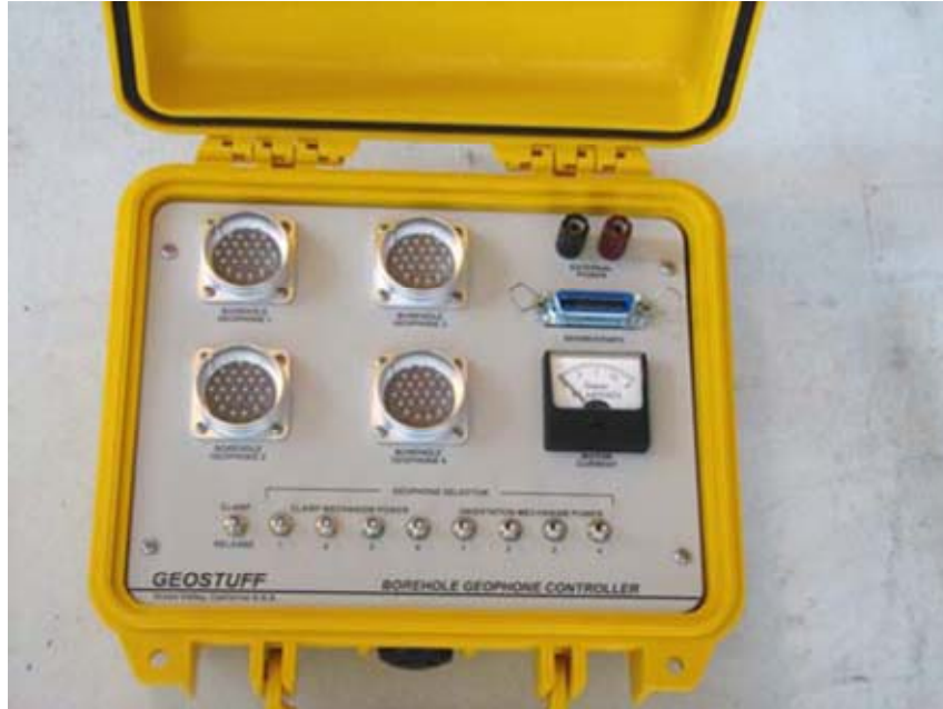
Figure 4.20 BHGC-4 Borehole geophone controller.
