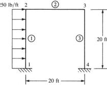
2. For the ridge frame shown below, determine the displacements and rotations at the nodes, the element forces, and the reactions (Problem 5.28).
