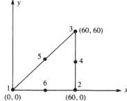
5. For the element show below subjected to the linearly varying line load acting over the vertical side, determine the nodal force replacement system. Compare the results to those obtained for a same load acting over a CST element (Problem 8.4).
