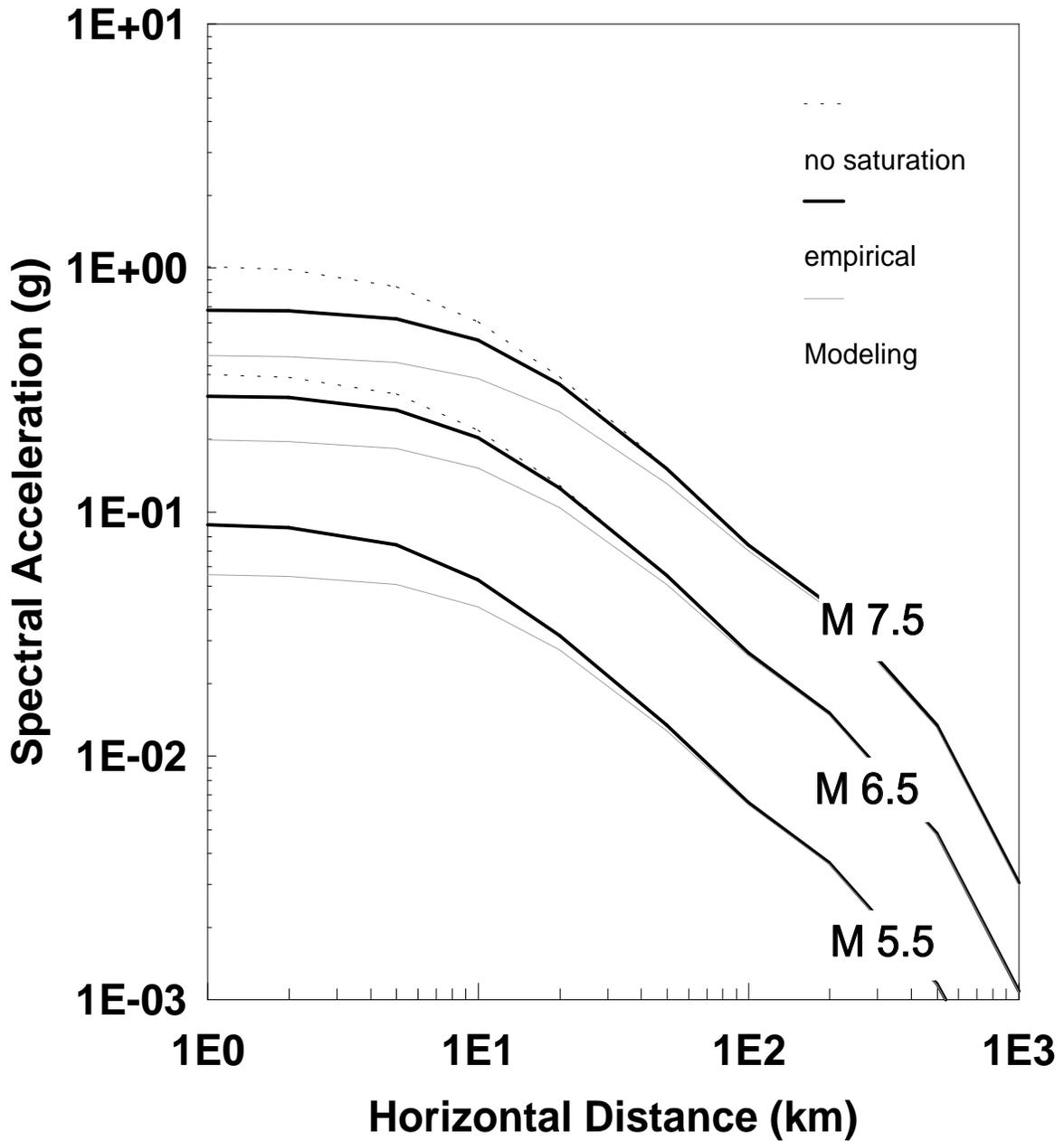
Figure 4-5. Median extended-source attenuation equations for 1-Hz spectral acceleration.. Note: the no-saturation and empirical predictions for M 5.5 are identical.
