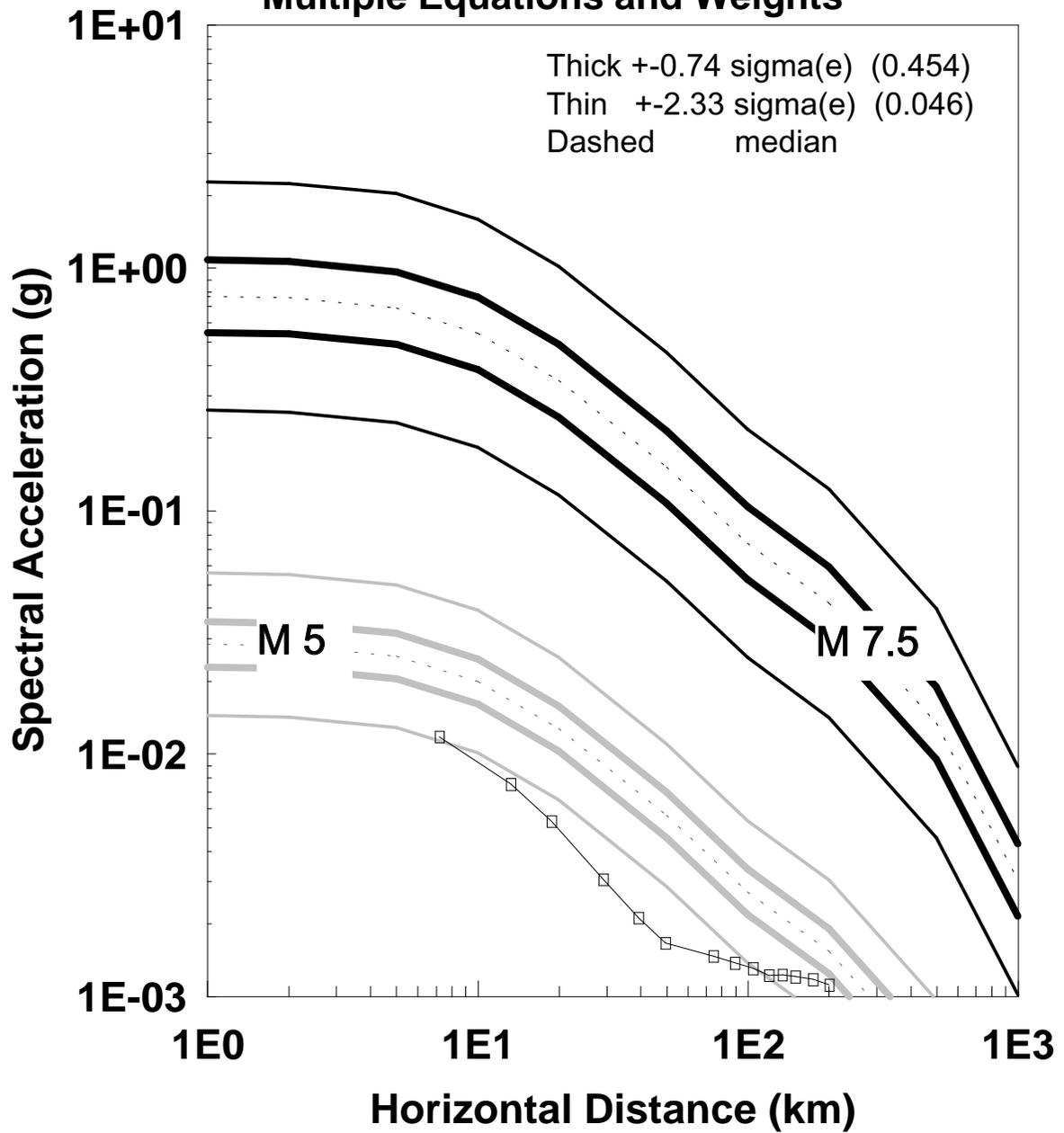
Figure 4-2. EPRI attenuation equations for 1-Hz spectral acceleration on rock (point-source assumption).
