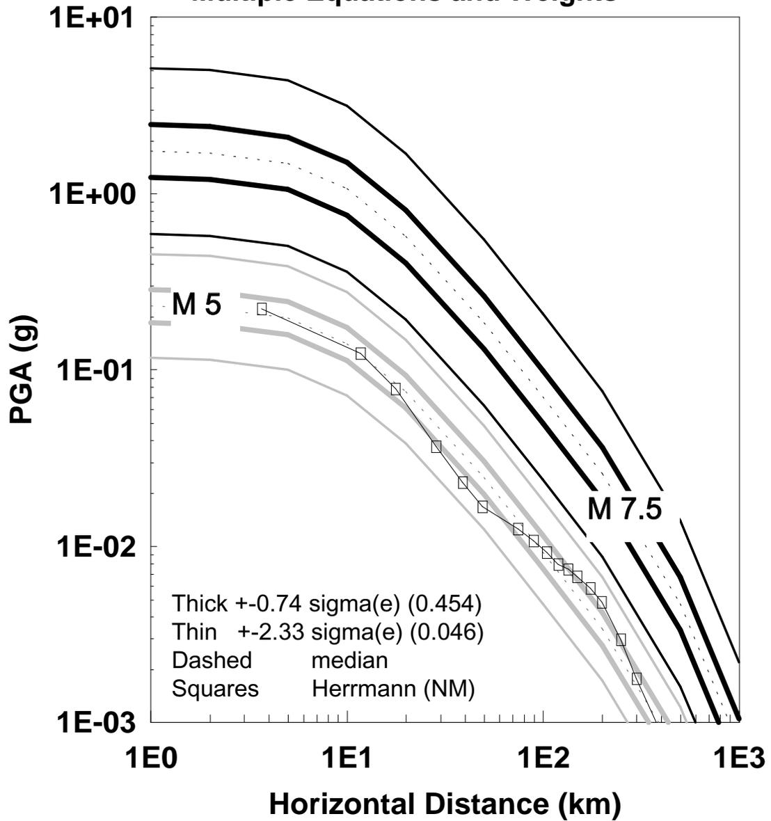
Figure 4-1. EPRI attenuation equations for PGA on rock (point-source assumption).
