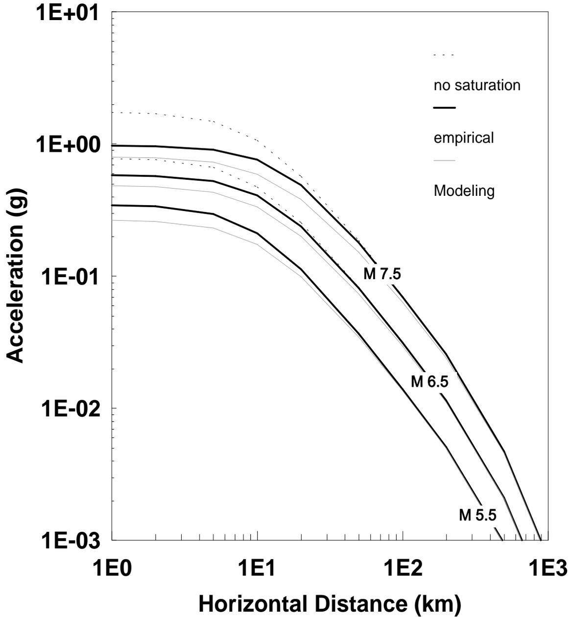
Figure 4-4. Median extended-source attenuation equations for PGA. Note: the no-saturation and empirical predictions for M 5.5 are identical.
