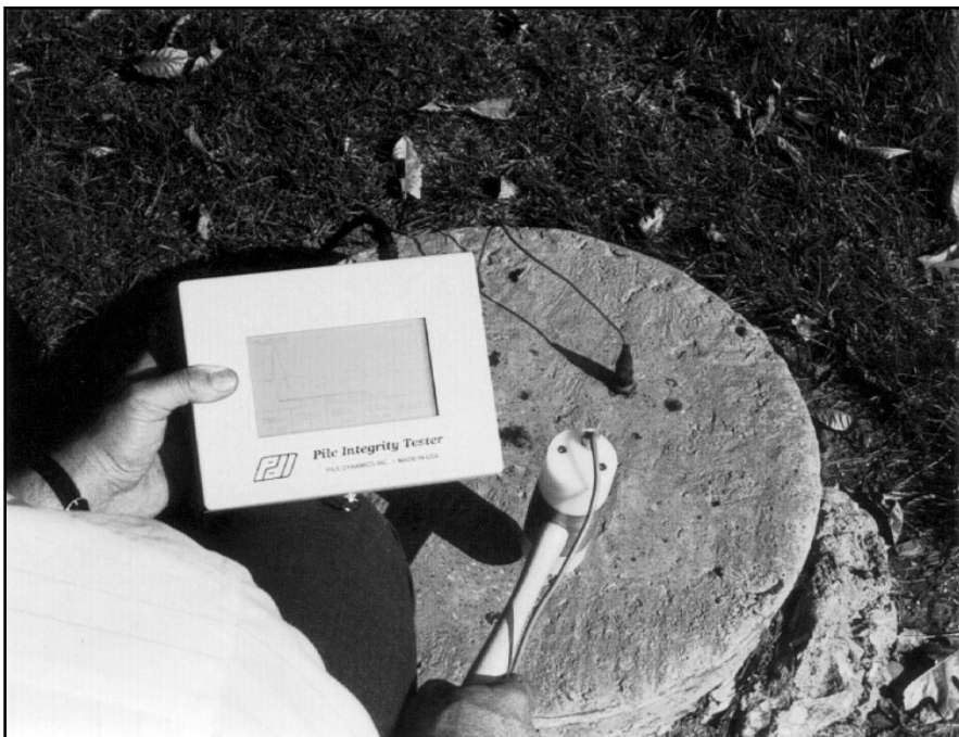
Figure 4243, Pile Integrity Tester (After PDI, 1993)
