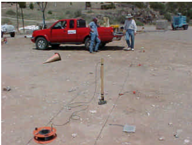
Figure 1. Combined ReMi and seismic refraction setup in Sandia Mountains, NM. Equipment is set up on the back of the truck. Geophone spacing is 10 feet and the array length is 120 feet. The author is beginning to jog to generate surface waves for a ReMi data set; the sledgehammer seismic refraction energy source is in the foreground.
