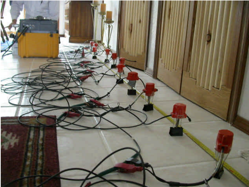
Figure 8. Small scale ReMi array setup to evaluate fill conditions under concrete slab. Binder clips were set on spikes and then taped to the geophone bodies for mounting on the floor.
