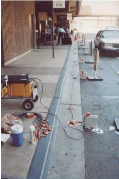
Figure 3. Typical field setup for ReMi data collection along loading and unloading curbs at airport terminals. Note cinder blocks used to assist with geophone placement on pavement. Geophones were placed on hollow cinder blocks set on the pavement in a 12-geophone array with 10-foot spacing. Each ReMi data set was 12 seconds long at 1 millisecond sample intervals. Twenty-eight Hz geophones are set up on the cinder blocks, and 4.5 Hz geophones are collected on the sidewalk next to the seismograph. The ReMi test is being performed on a street section consisting of a minimum of 5-inches of asphaltic concrete pavement over an aggregate base course. Although the site was hopelessly noisy for seismic refraction as well as being paved, the ambient noise served well as a source for the ReMi method.
