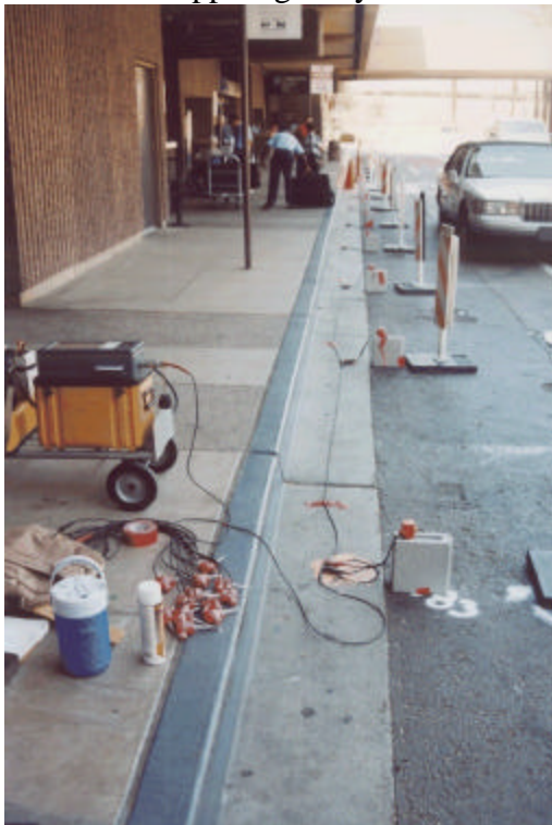
Figure 2. Typical field setup for ReMi data collection along loading and unloading curbs at airport terminals. Note cinder blocks used to assist with geophone placement on pavement. Geophones were placed on hollow cinder blocks set on the pavement in a 12-geophone array with 10-foot spacing. Each ReMi data set was 12 seconds long at 1 millisecond sample intervals. Twenty-eight Hz geophones are set up on the cinder blocks, and 4.5 Hz geophones are collected on the sidewalk next to the seismograph. The ReMi test is being performed on a street section consisting of a minimum of 5-inches of asphaltic concrete pavement over an aggregate base course. Although the site was hopelessly noisy for seismic refraction, as well as being paved, the ambient noise served well as a source for the ReMi method.
