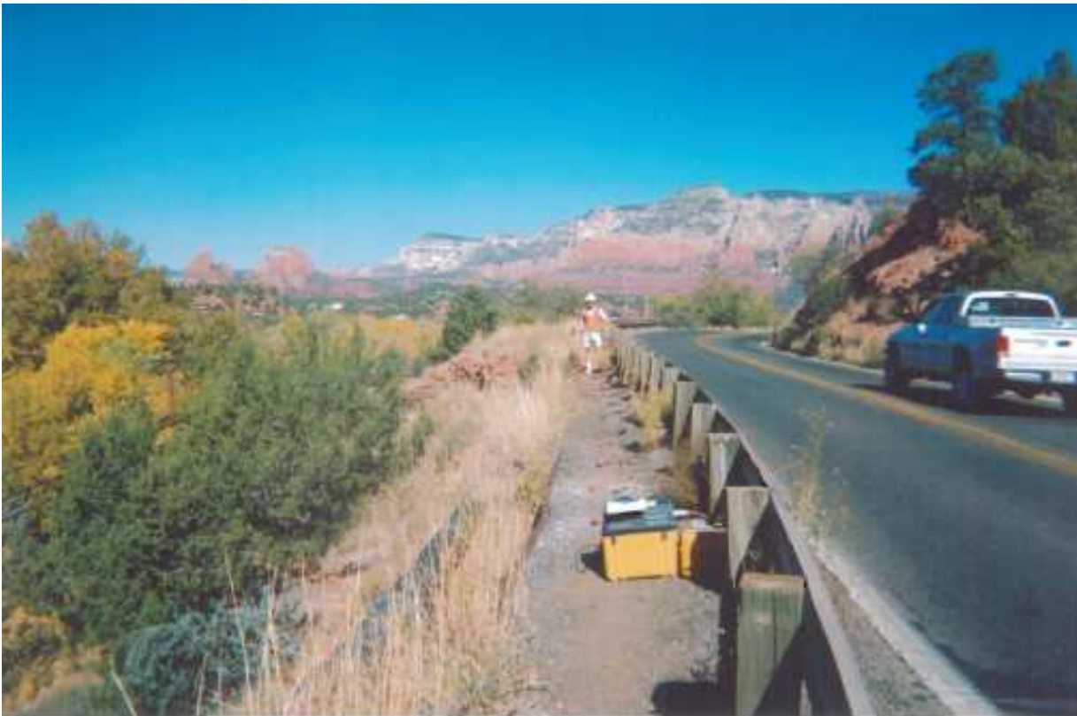
Figure 2. Field setup for p- and s-wave data collection to assess the subsurface profile for highway SR 179 improvements in Sedona, Arizona along a difficult access sidehill cut and fill using a 12-channel seismograph. A 60 foot (18 m) long 12 geophone array is deployed using a 120 foot (36 m) geophone cable. A 10-lb (4.5 kg) sledgehammer with trigger switch and cable is the p-wave energy source. Traffic on the highway and the operator jogging are ambient s-wave energy sources. Battery, geophones, notebook and other field items are carried by backpack. Drill rig access was not feasible here both due to limited space and the presence of buried utilities in the fill portion of the existing side-hill cut and fill section. Multiple seismic lines were completed end to end to obtain a continuous profile in this area.
