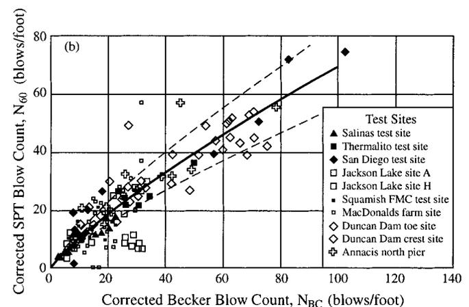
FIG. 10. Correlation between Corrected Becker Penetration Resistance  $N_{BC}$  and Corrected SPT Resistance  $N_{60}$ : (a) Harder and Seed (1986); (b) Data from Additional Sites (Reproduced from Harder 1997)
