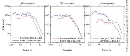
Figure 9. Spectra at LEXD and LGPC.
