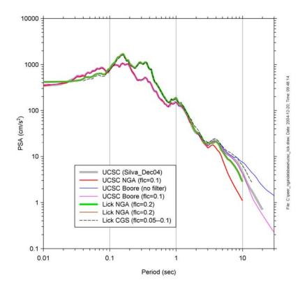
Figure 1. Spectra of data recorded on the UCSC campus. The new spectrum at UCSC (gray) is in good agreement with my spectrum of filtered motion (magenta). Note that the difference between the Lick and UCSC spectra is probably real.
