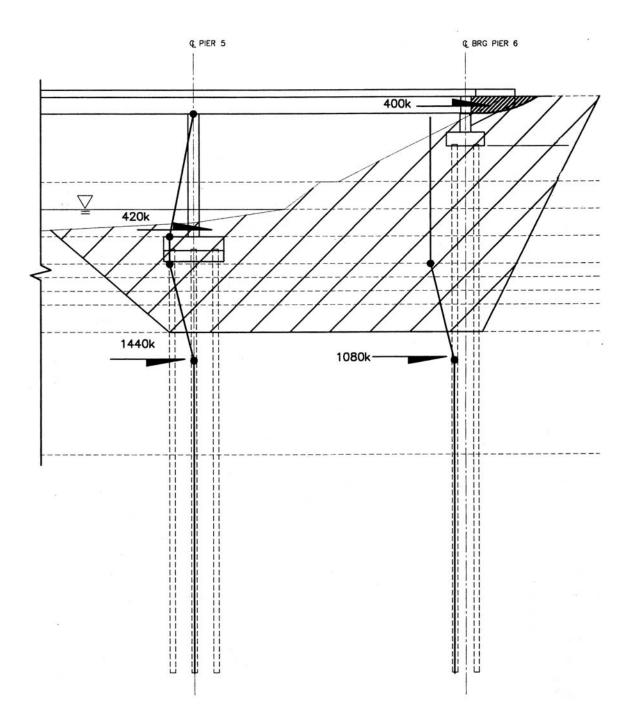
Figure 4: Foundation Movements and Resisting Forces from Lateral Spreading
