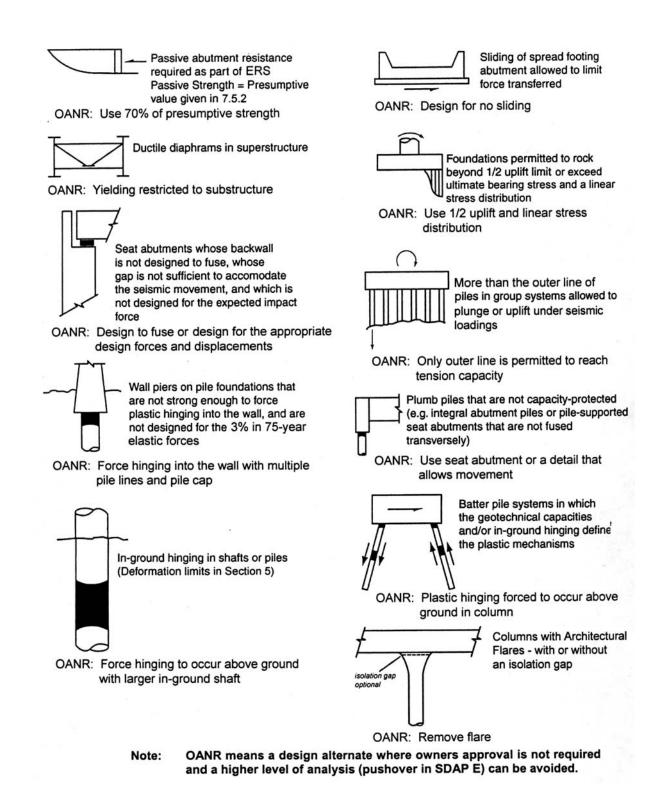
Figure 3: Earthquake Resisting Elements (ERE) that Require Owner's Approval
