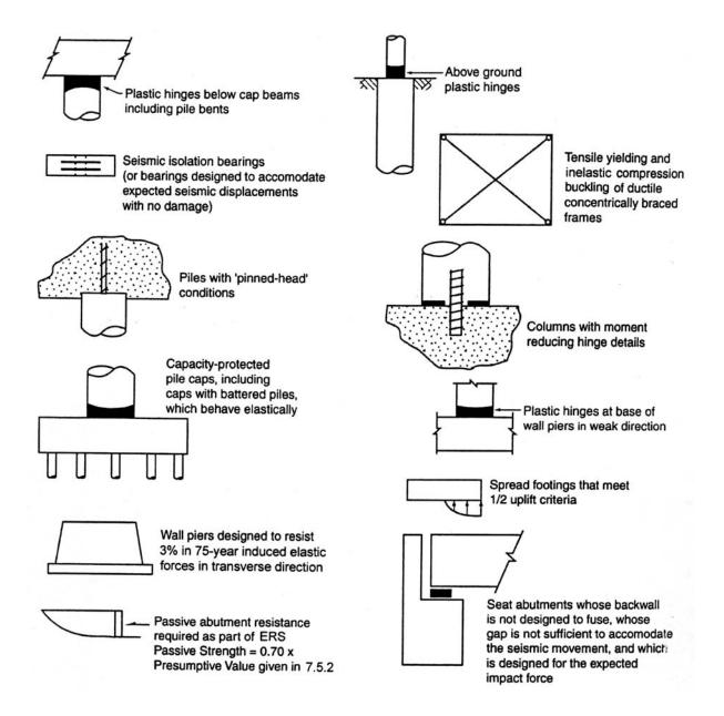
Figure 2: Permissible Earthquake Resisting Elements (ERE)
