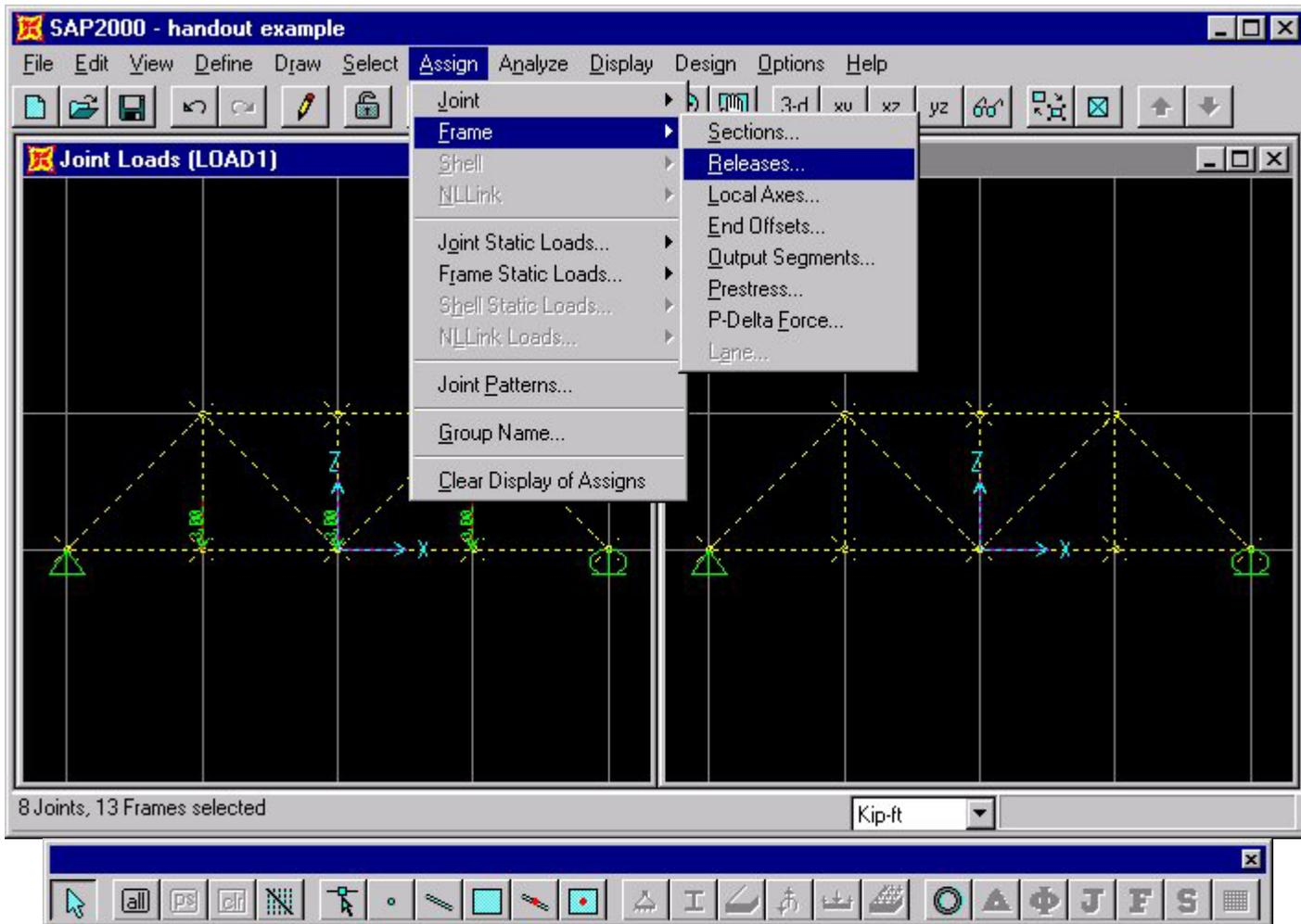
In this example, the structure is a truss, which by definition has no moment capacity at each joint. To release the moment capacity, click on the check boxes that are associated with the **Moment 22**, **Moment 33**, and **Torsion**. Torsion can only be released at one end of the element, whereas, the other moment must be released at both the **Start** and **End** of the element.
