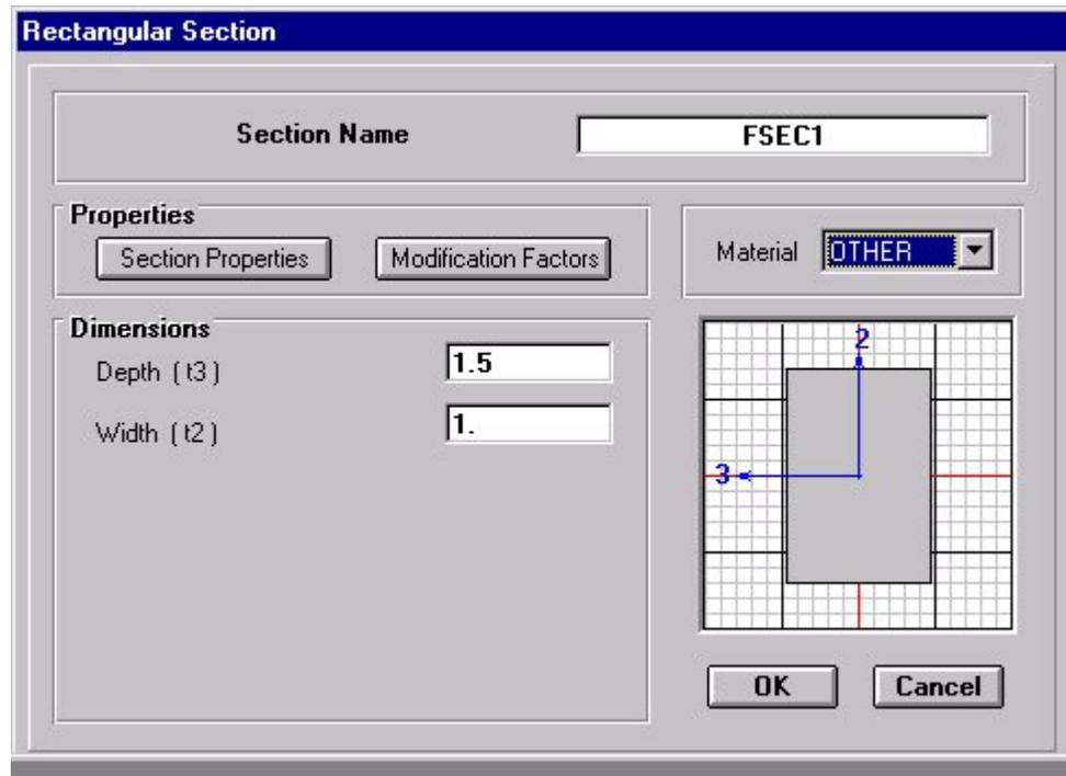
To the material of this frame section click on the **Material** pull-down menu and select our weightless material **OTHER**. Click **OK** to return to the **Define Frame Sections** window and then click **OK** again. If you are interested in computing deflections in the truss, then you must define the Depth (t3) and Width (t2) of the cross-section. In this example, we are interested only in the axial forces in a determinate truss, so the value of the cross-sectional areas are not important.
