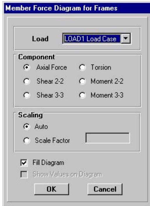
The default values will display the **Axial Forces** using the **Fill Diagram**. If you click OK, the SAP 2000 interface window will display the relative magnitude of the axial forces with compress forces in **red** and tension forces in **yellow**.
