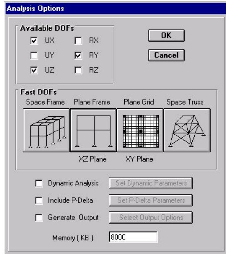
To restrict SAP 2000 to variables in the x- plane, select the **Plane Frame** button and click **OK**. The truss structure is now ready for analysis. To analyze the model press the **Run Analysis** button
