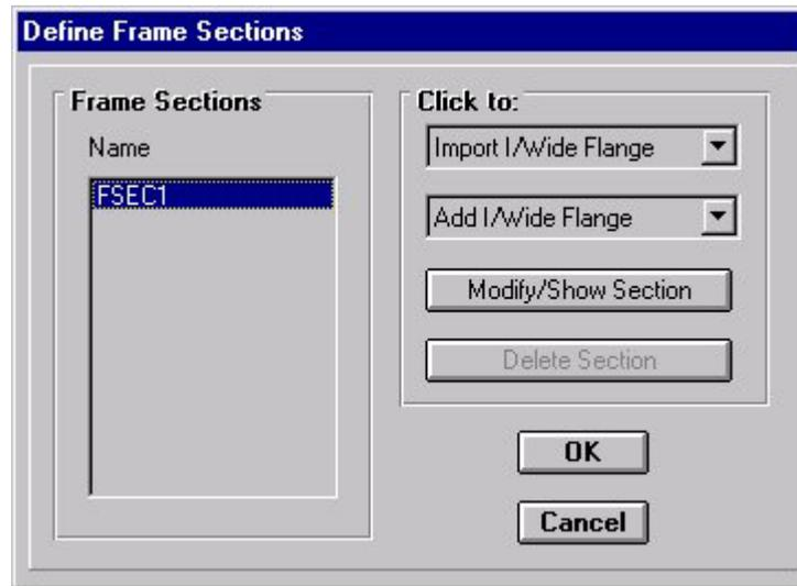
The default Frame Section label is **FSEC1**. To change the properties of the frame section click on the **Modify/Show Material** button. The **Rectangular Section** window will appear.
