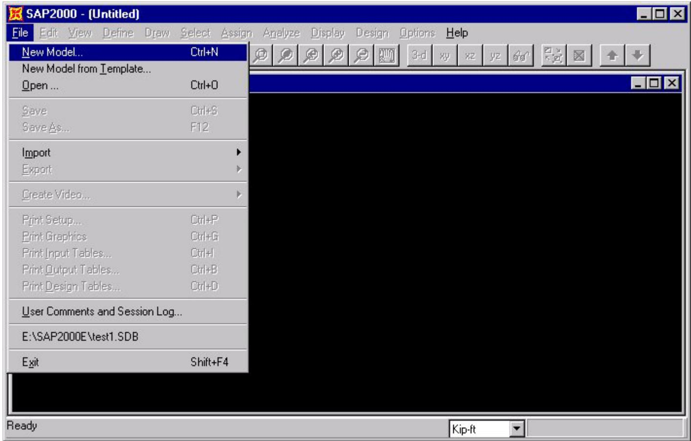
When you select **New Model** on the menu, the **Coordinate System Definition** window will appear (see the figure on the right).
