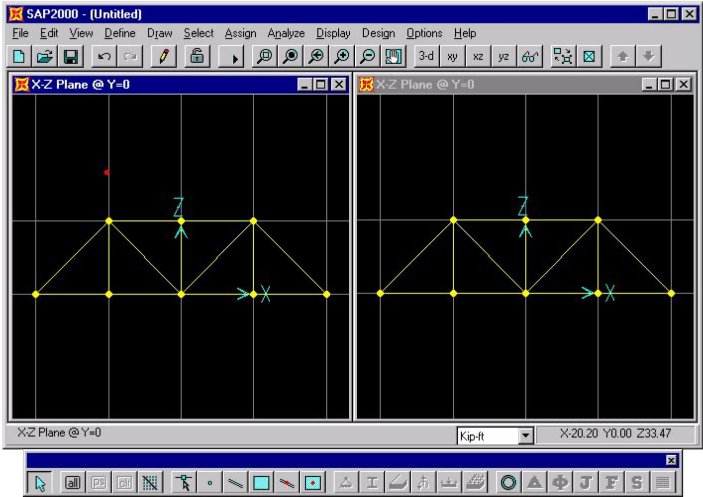
**Step 5: Define Structural Supports** - To define the location and type of structural support, select the support location by clicking on the joint with the pointer. A yellow "X" should appear at the joint to indicate that it is currently selected. Next click on the **Joint Restraint** button
