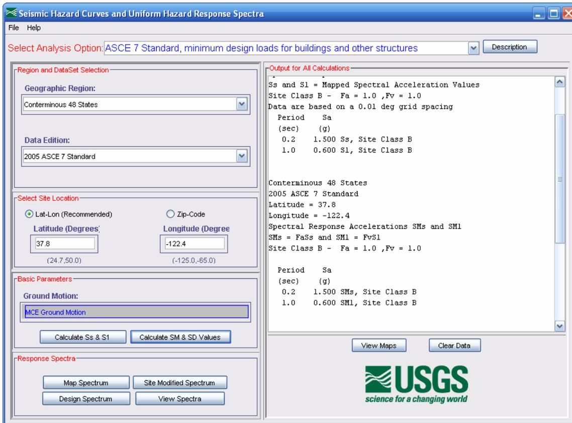
Figure 5-3 Data input to USGS ground motion calculator to generate a response spectrum
