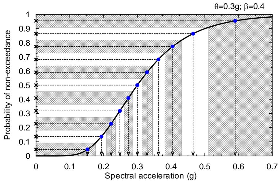
Figure 5-6 Calculation of spectral accelerations given a lognormal distribution
