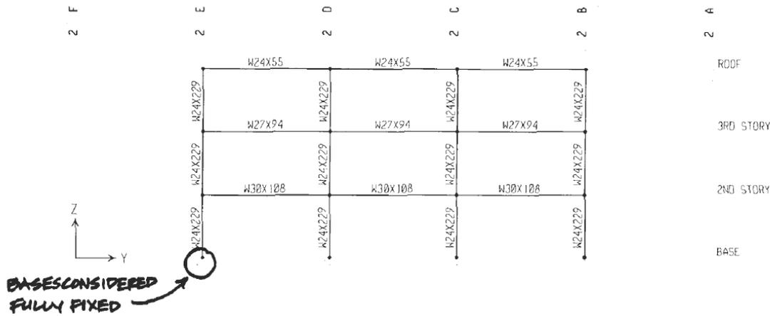
Figure 7-3 Elevation of typical steel moment frame for example building (no scale)
