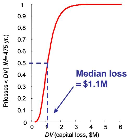
Figure 2-1 Cumulative loss function identifying a median (50th percentile) loss
