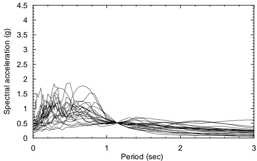
Figure 7-4 Spectral accelerations for Bin I ground motions
