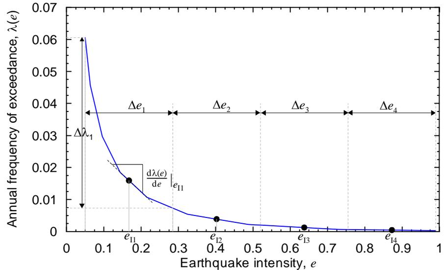
Figure 3-7 Seismic hazard curve and time-based loss calculations
