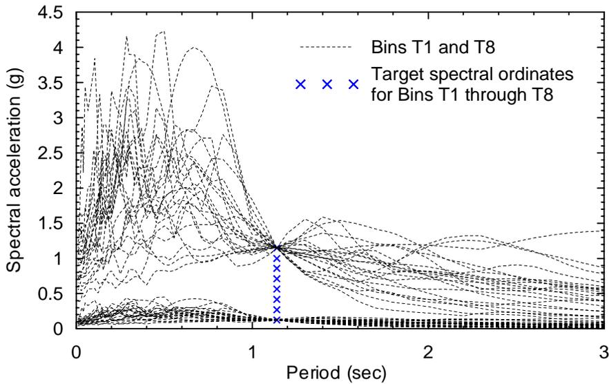
Figure 7-12 Target spectral ordinates for Bins T1 through T8 and spectra for scaled ground motions in Bins T1 and T8
