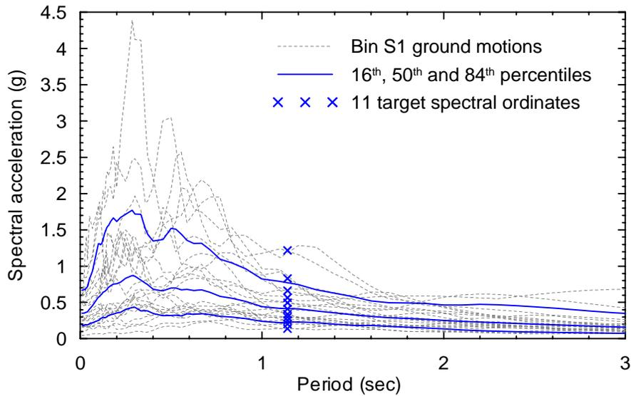
Figure 7-6 Spectral accelerations for Bin S1 ground motions, 16<sup>th</sup>, 50<sup>th</sup> and 84<sup>th</sup> percentiles of spectral acceleration and the 11 target spectral ordinates for Bin S1 motions
