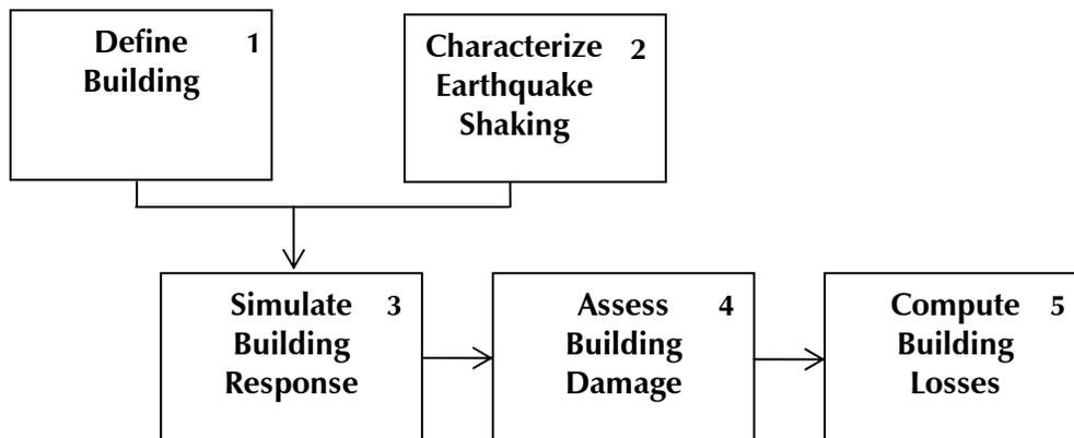
Figure 3-1 Procedure for Seismic Performance Assessment
