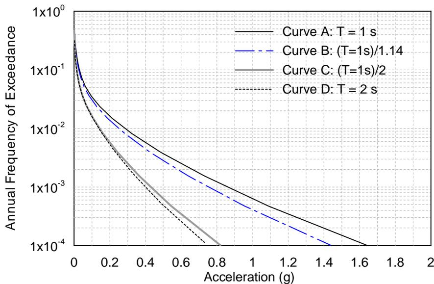
Figure 7-10 Seismic hazard curves for the site of the building
