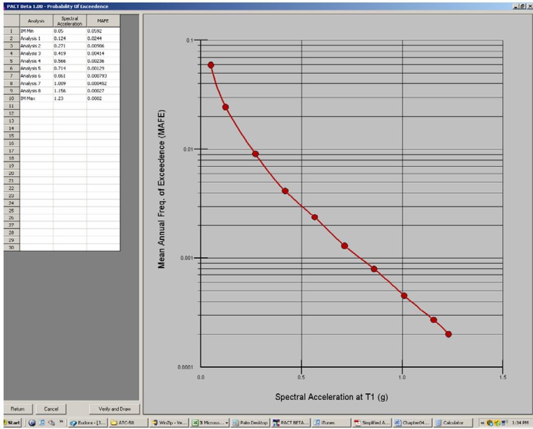
Figure 4-5 Sample seismic hazard curve in PACT
