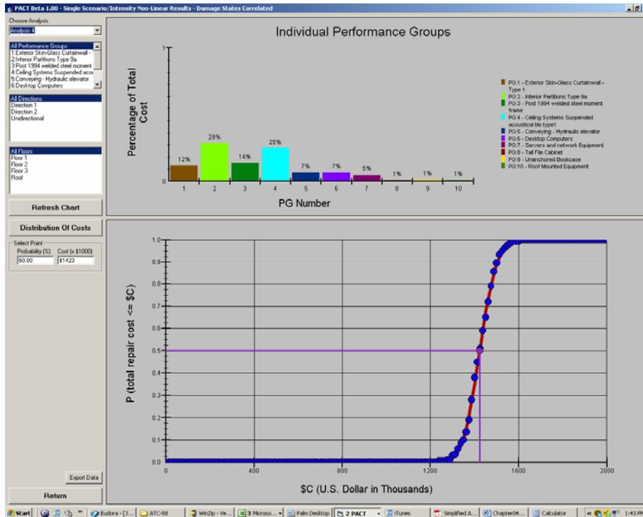
Figure 4-10 Sample loss calculations from PACT for a scenario or intensity-based assessment.
