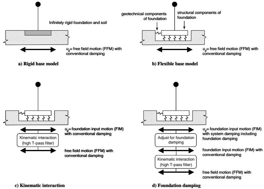
Figure B-9 Analysis for soil foundation structure interaction (FEMA, 2005)
