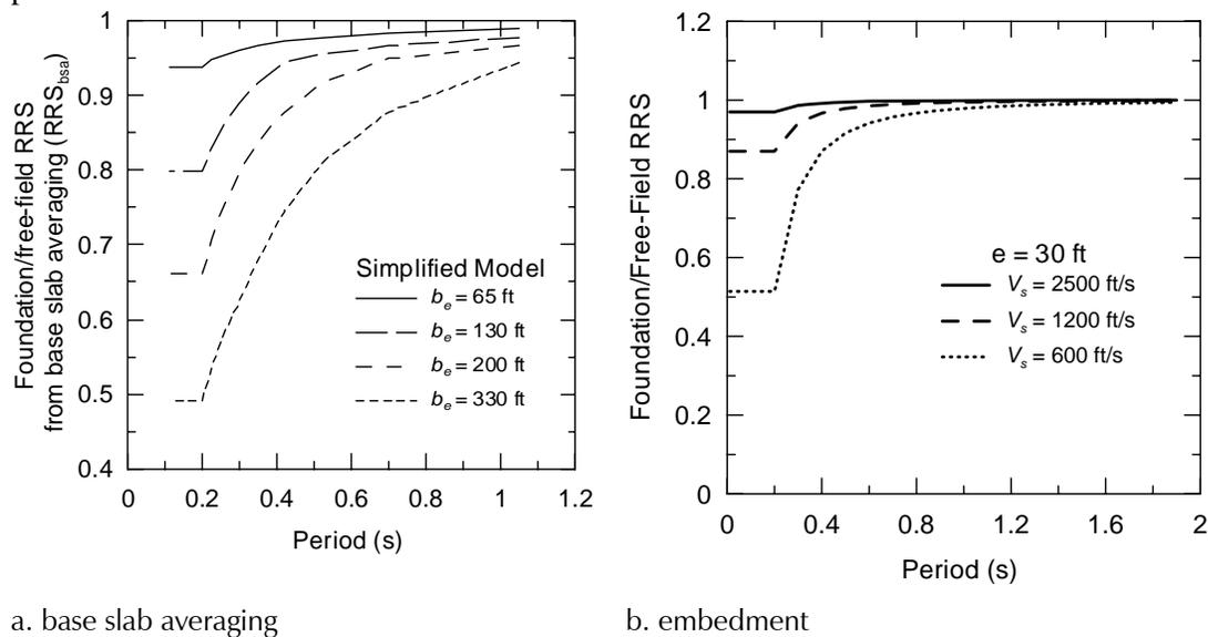
Figure B-10 Reductions in spectral demand due to kinematic interaction
