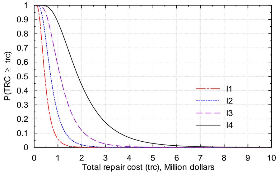
Figure 3-2 Example cumulative probability distributions for loss exceeding a specified value for a hypothetical building at four ground motion intensities
