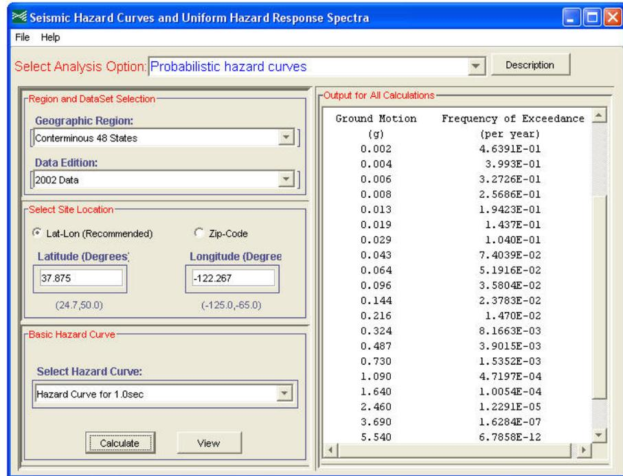
Figure 7-8 Screen capture from USGS ground motion calculator for generating a one-second hazard curve for the site of the building
