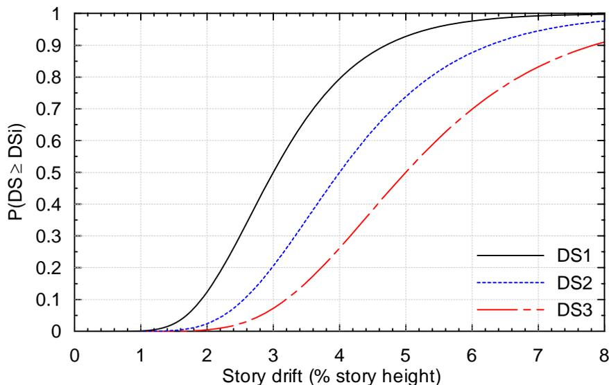
Figure 3-5 Example family of fragility curves for special steel moment frames
