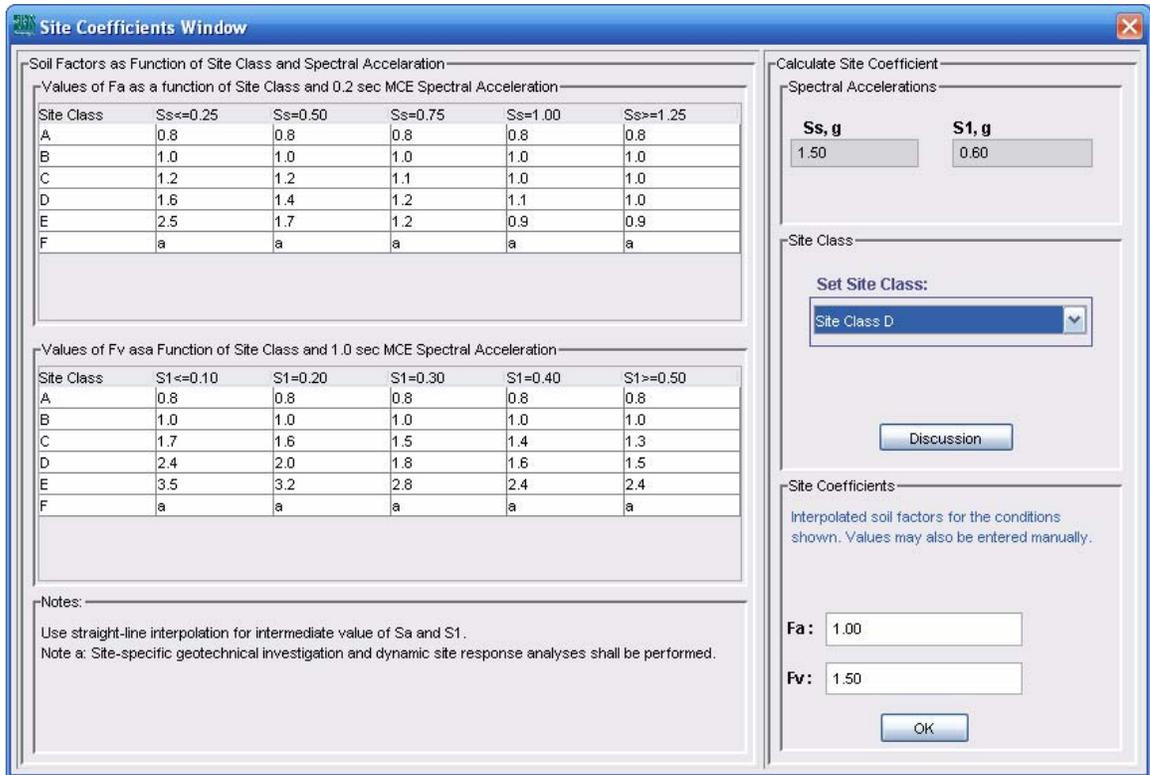
Figure 5-4 Data input to USGS ground motion calculator to modify the response spectrum for non-reference soil conditions
