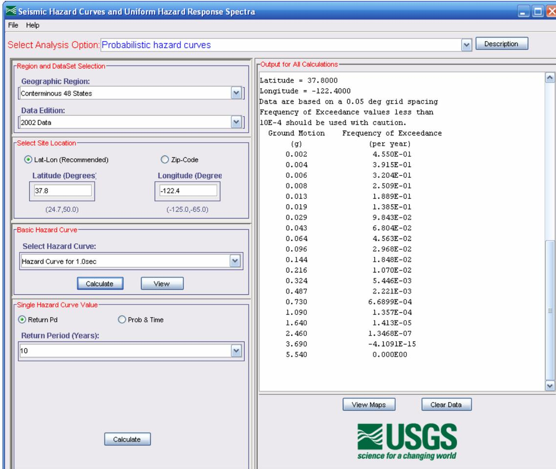
Figure 5-1 Screen capture from the USGS ground motion calculator
