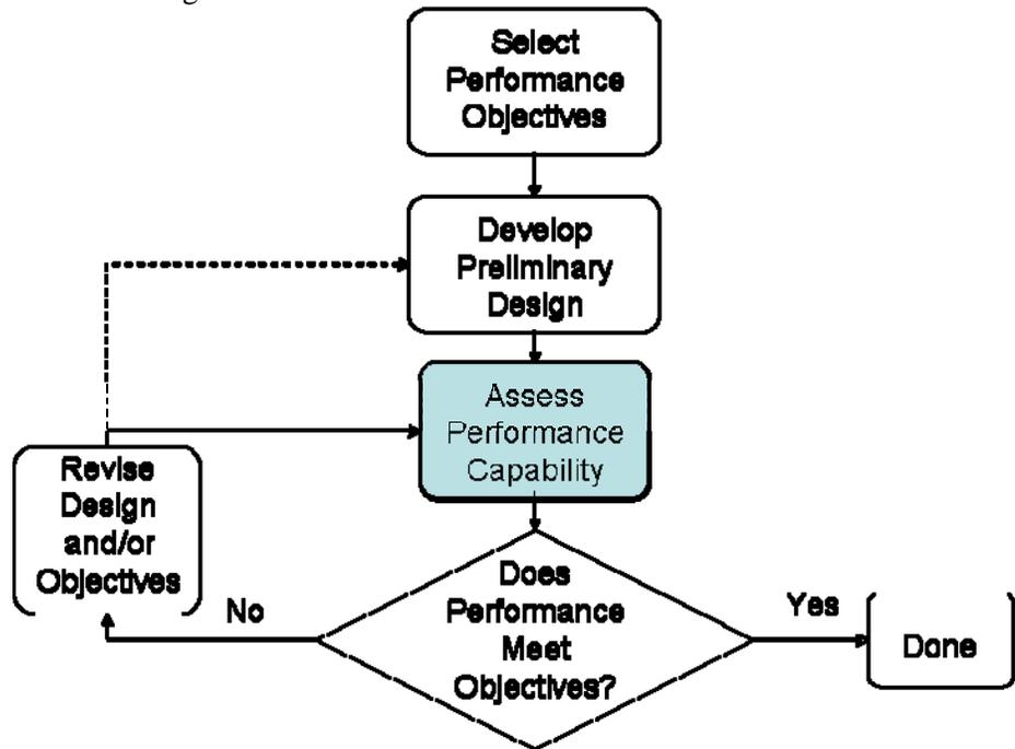
Figure 1-1 Performance-based design flow diagram
