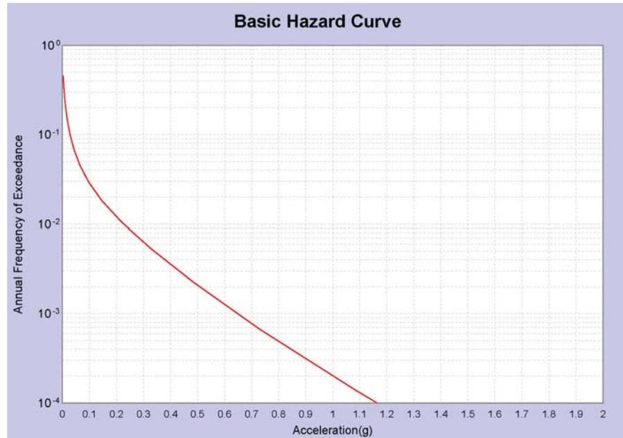
Figure 5-2 Hazard curve for data shown in Figure 5-1, plot in log-linear format
