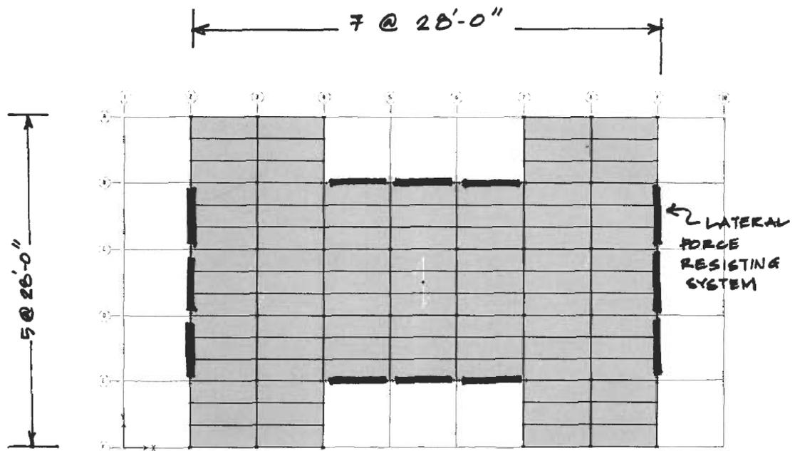
Figure 7-2 Schematic structural framing plan for example building (no scale)
