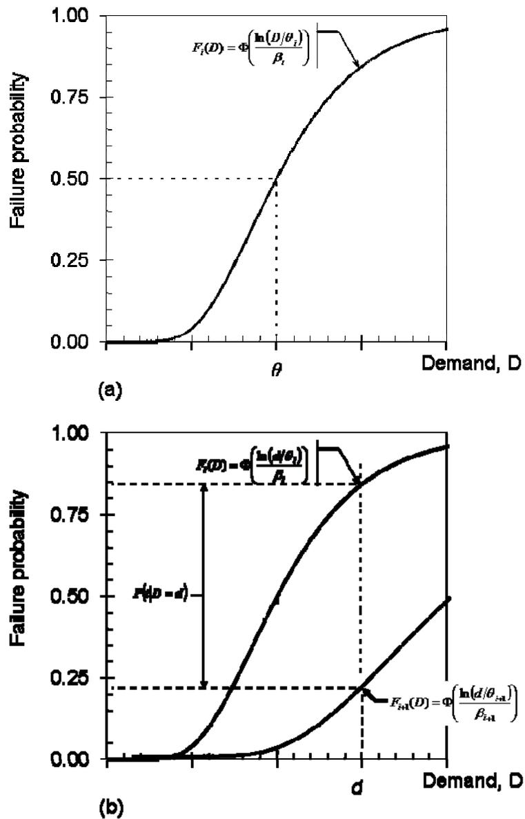
Figure C-1 Illustration of (a) fragility function, and (b) evaluating individual damage-state probabilities
