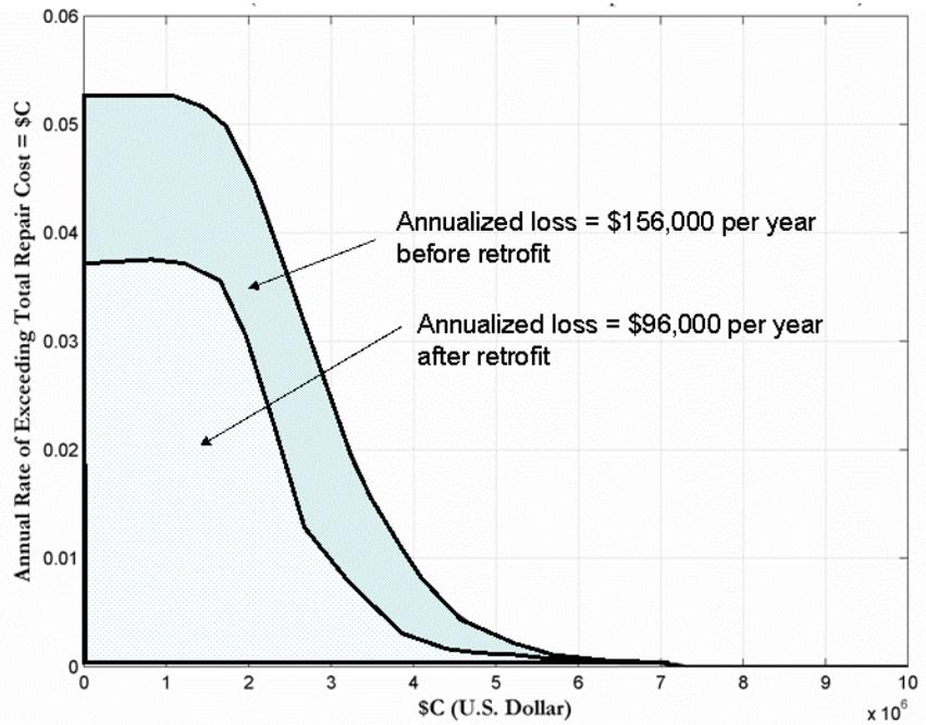
Figure 2-4 Annualized loss before and after proposed retrofit
