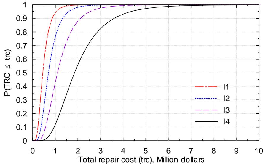
Figure 3-3 Example cumulative probability distributions for loss less than a specified value for a hypothetical building at four ground motion intensities
