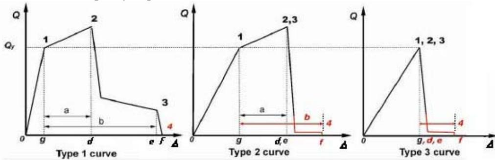
Figure 6-1 Generalized force-displacement behavior of structural components
