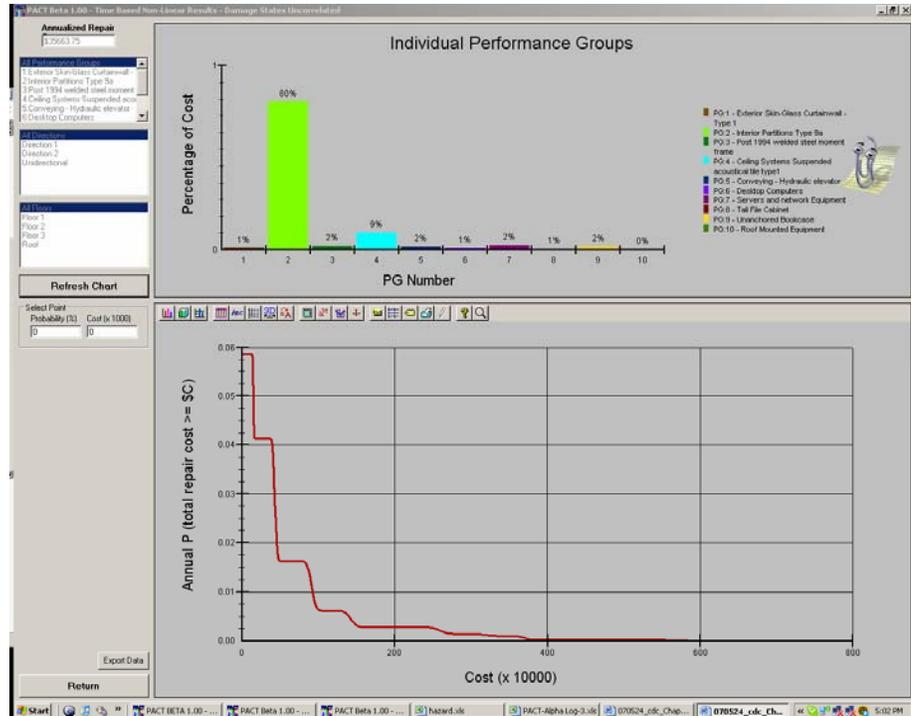
Figure 4-11 Sample loss calculations from PACT for a time-based assessment.
