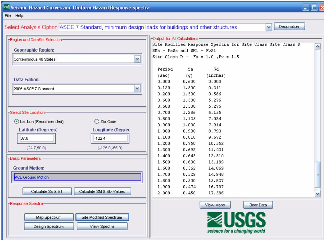
Figure 5-5 Sample response spectrum calculation for an intensity-based assessment
