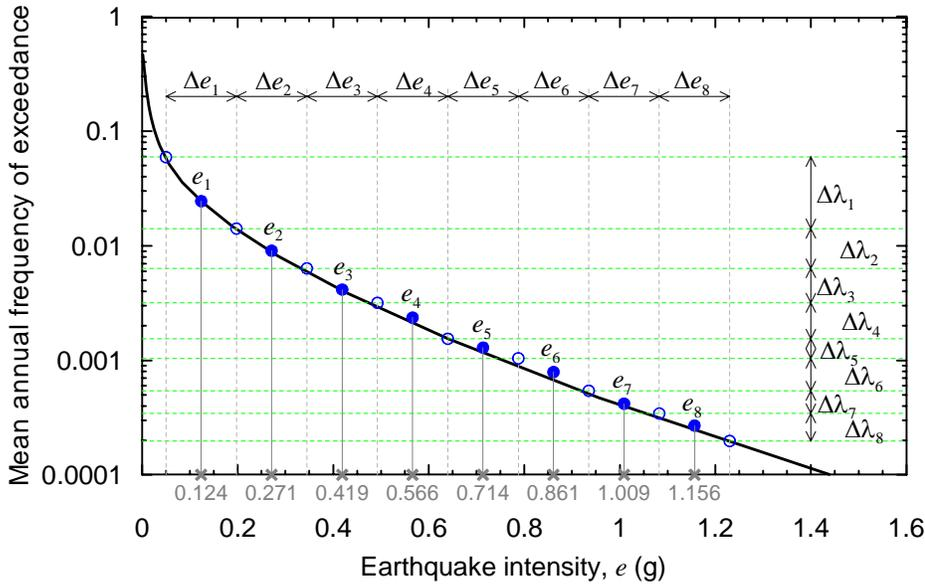
Figure 7-11 Characterizing seismic hazard for time-based assessment
