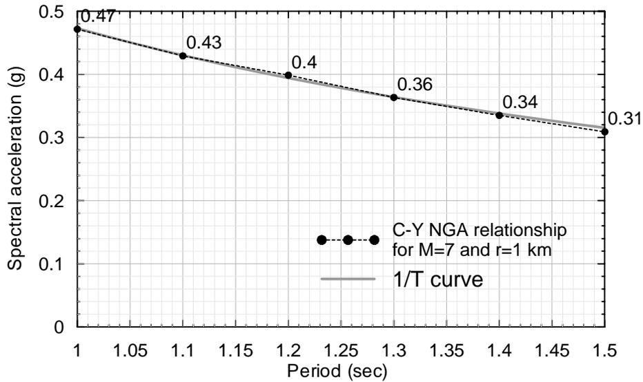
Figure 7-5 Spectral accelerations per the Chiou-Youngs NGA relationship for  $M_w = 7$ ,  $r = 1$  km, strike-slip faulting and  $v_{30} = 760$  m/s, and varying as  $0.47/T$
