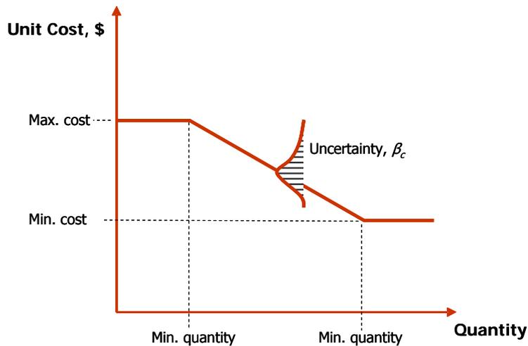
Figure 3-6 Sample consequence function for cost of repair
