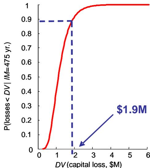
Figure 2-2 Illustration of Probable Maximum Loss (PML)
