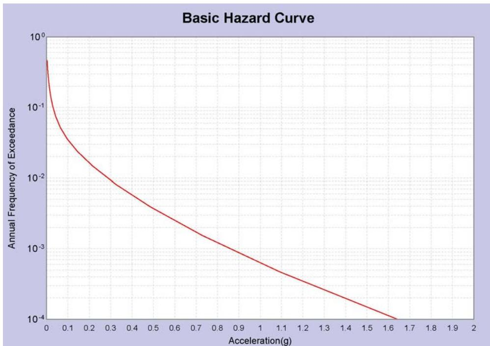
Figure 7-9 One-second seismic hazard curve
