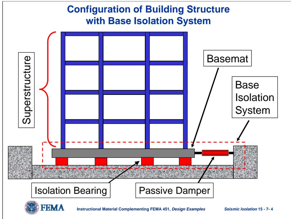
The basic elements of a base isolation system are shown in this slide. Supplemental dampers may or may not be utilized within an isolation system.
