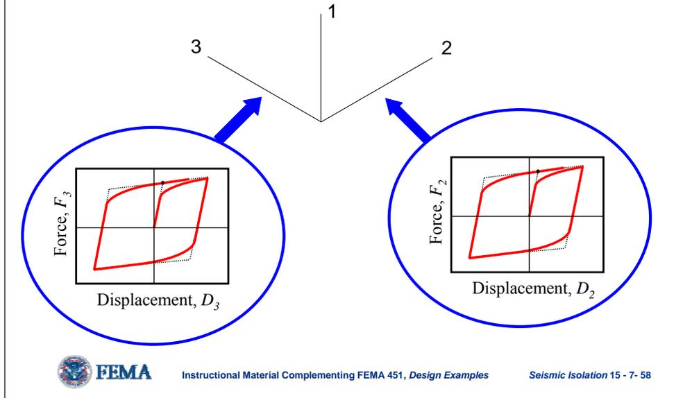
The ISOLATOR1 Property of the SAP2000 NLLINK element can be used to model a biaxial hysteretic isolation bearing. This element is well-suited to modeling the behavior of elastomeric bearings.
