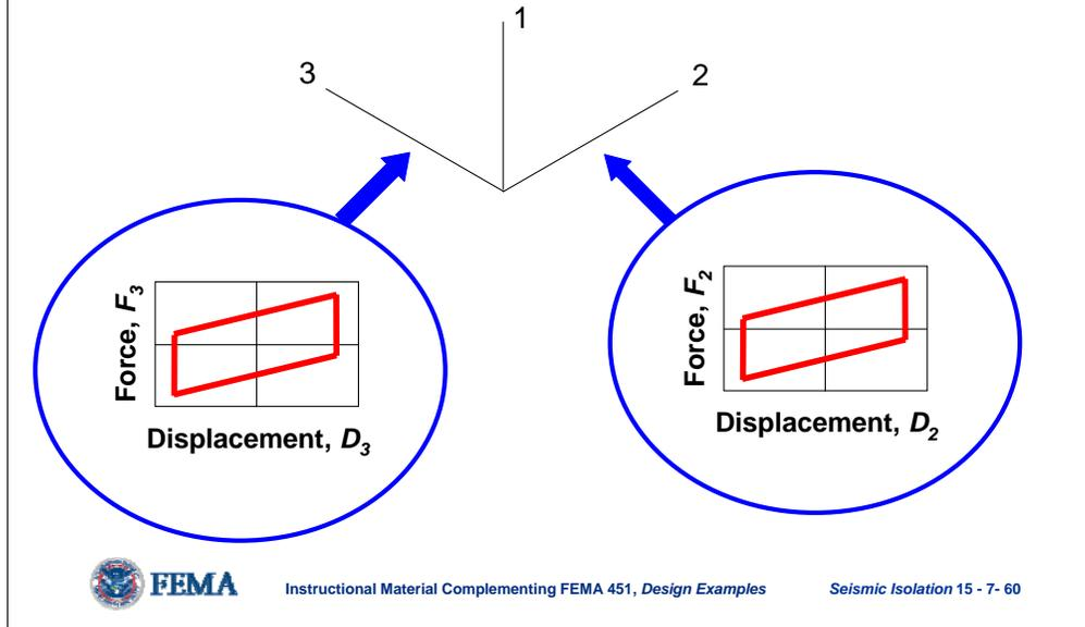
The ISOLATOR2 Property of the SAP2000 NLLINK element can be used to model a biaxial Friction Pendulum System isolation bearing.
