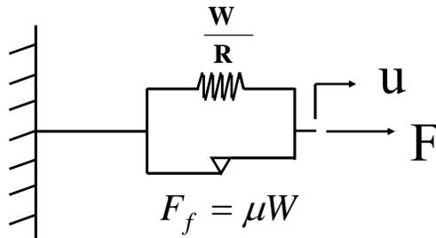
**Rigid Model with Strain Hardening**
