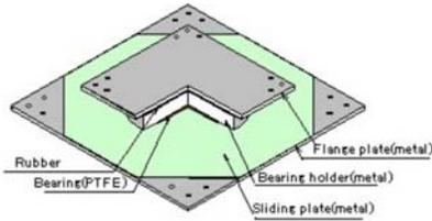
For Spherical Bearings:
