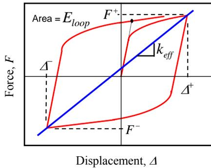
$$k_{eff} = \frac{|F^+| + |F^-|}{|\Delta^+| + |\Delta^-|} \quad \text{Effective Stiffness of Isolation Bearing}$$
