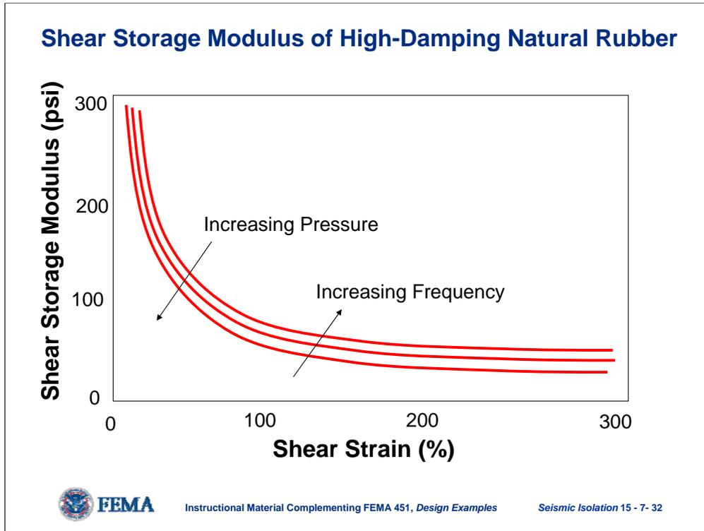
The stiffness of high damping rubber bearings decreases with increasing shear strain (and, then, although not shown here, increases again at higher shear strains). The increased stiffness at high shear strains is sometimes regarded as a fail-safe mechanism.
