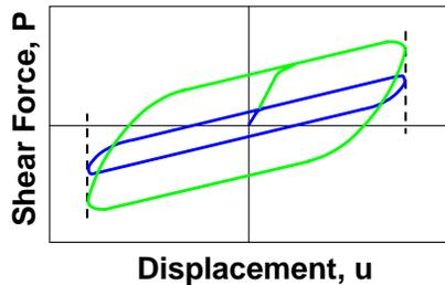
$k_{eff}$  = Effective stiffness at design displacement
