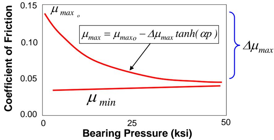
Figure is based on studies of PTFE-based self-lubricating composites used in FPS bearings.
