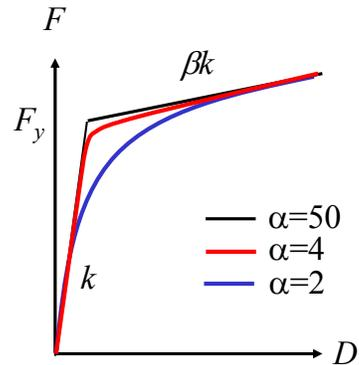
Note:  $Z$  is an internal hysteretic variable with magnitude less than or equal to unity. The yield surface is associated with a magnitude of unity.
