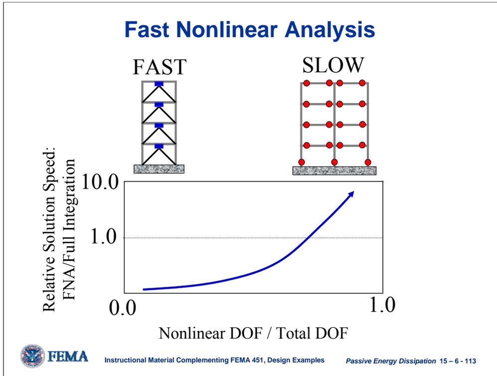
The Fast Nonlinear Analysis method is most efficient when the number of DOF associated with nonlinear behavior is small.
