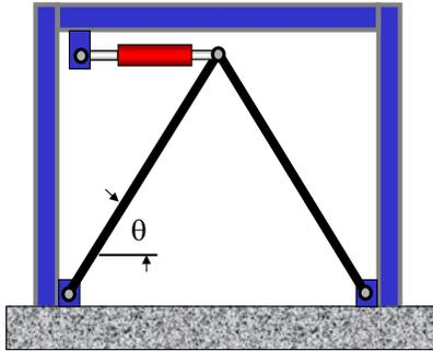
Because the damper is always in series with the linkage, the damper-brace assembly acts like a Maxwell model.
