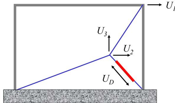
Displacement in Damper is *Out-of-Phase* with Displacement at DOF 1
