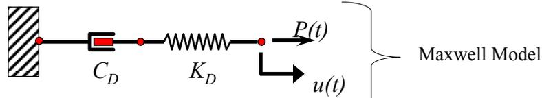
$$C(\bar{\omega}) = \frac{C_D}{1 + \lambda^2 \bar{\omega}^2}$$
