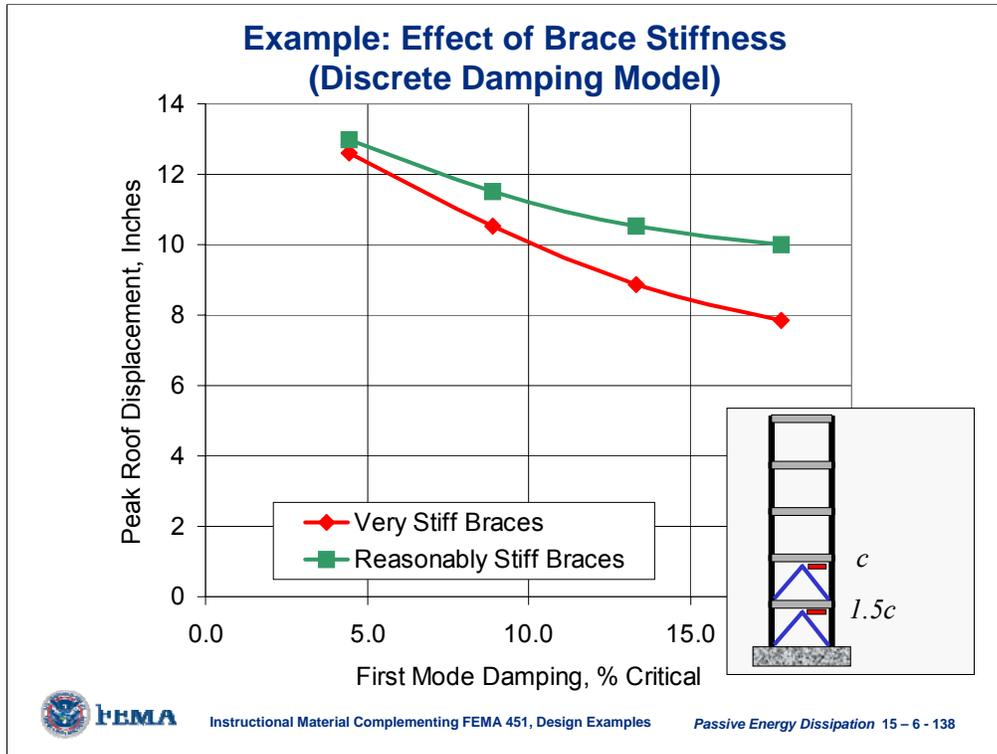
The peak roof displacement is larger if a realistic brace stiffness is used in the analysis. Thus, as expected, the effectiveness of the dampers is reduced due to the presence of the bracing. Since the potential benefit of high levels of damping are partially lost due to bracing flexibility, the influence of the brace stiffness on the roof displacement response is more significant for higher levels of damping.
