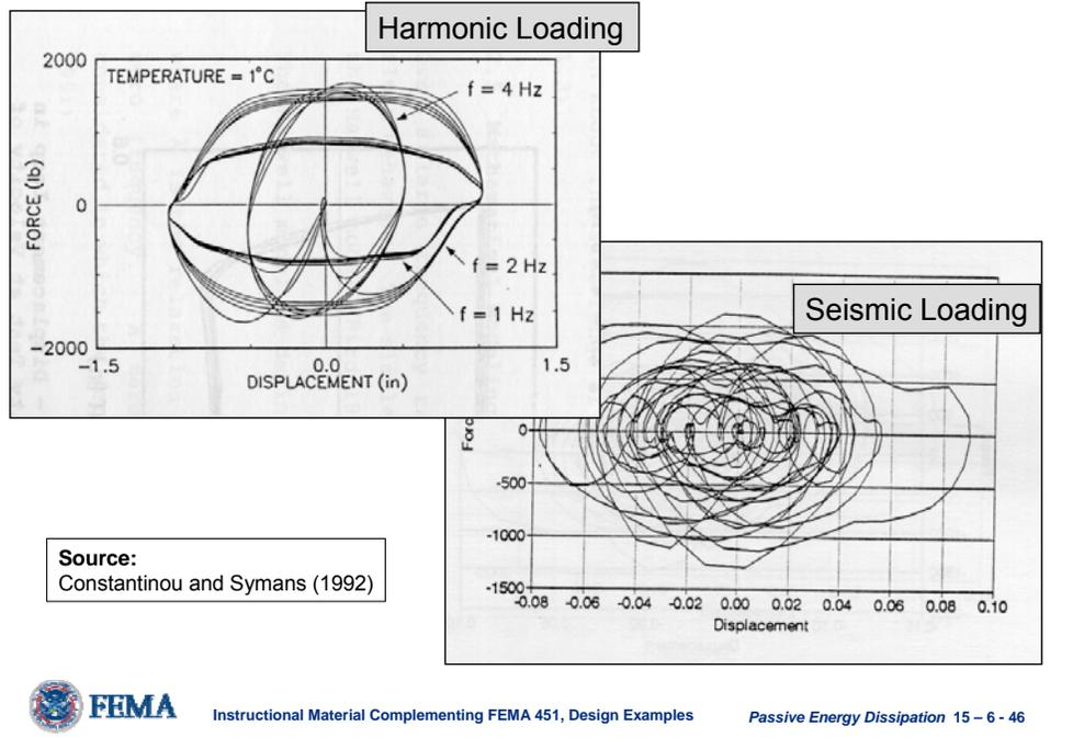
The hysteresis loops shown are for harmonic loading and seismic loading. The results from three different harmonic tests are shown. For each test, the loops are approximately elliptical in shape. The hysteresis loop for the seismic loading consists of a number of hysteresis loops, each of which is approximately elliptical in shape.
