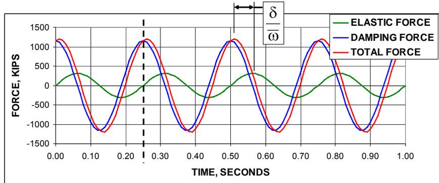
**Note: Damping force 90° out-of-phase with elastic force.**
