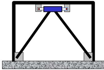
Dampers may be similarly modeled using the zero-length “Type-4” connection element.
