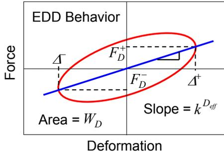
$$c_{eq} = 2m\omega_n \xi_{eq} = \frac{2m\omega_n W_D}{4\pi W_S} = \frac{W_D T}{2\pi^2 \Delta^2}$$
