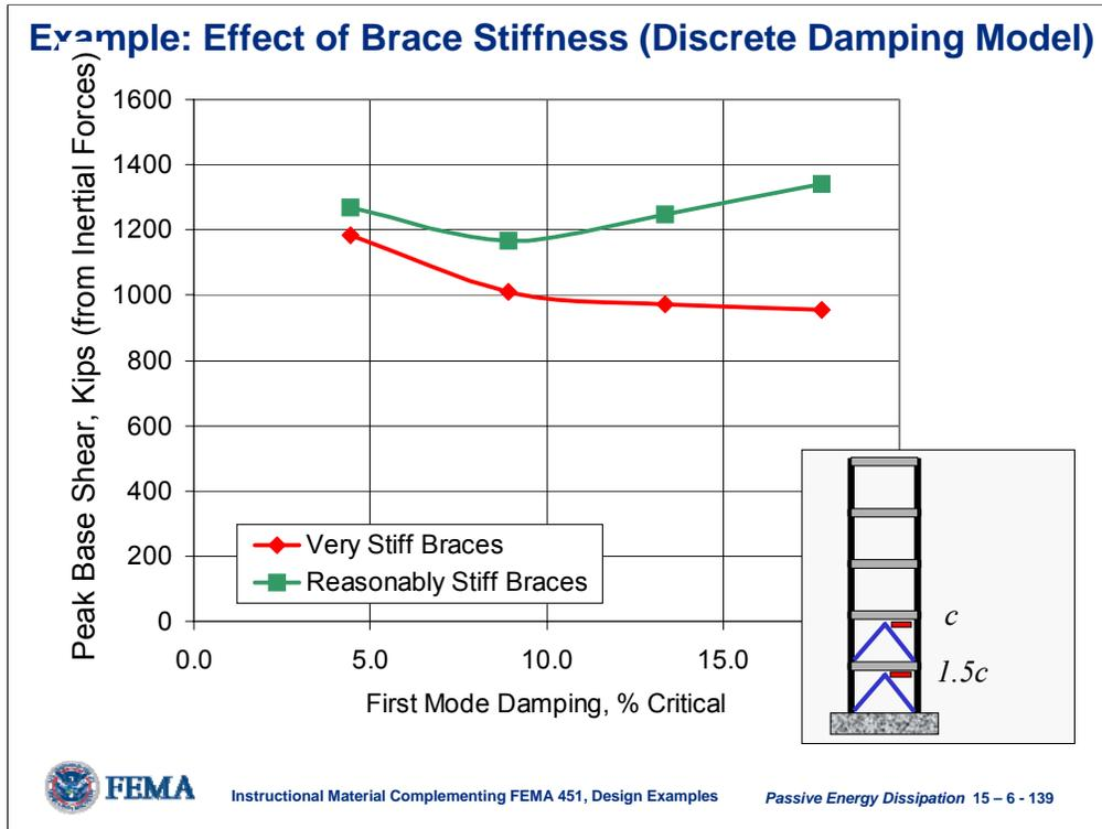
The peak base shear is larger if a realistic brace stiffness is used in the analysis. This is expected since, for realistic brace stiffness, the dampers are not as effective in limiting the lateral deformations of the structure and, in turn, the shear forces in the structure are increased. Since the potential benefit of high levels of damping are partially lost due to bracing flexibility, the influence of the brace stiffness on the base shear is more significant for higher levels of damping.
