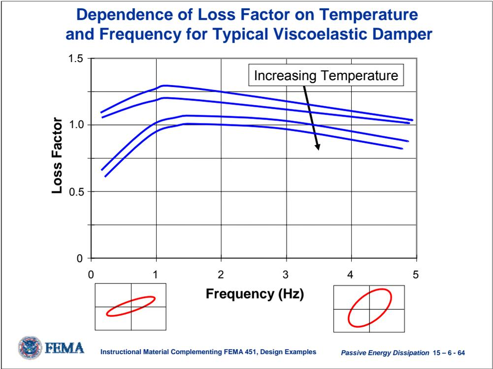
At a given frequency and strain amplitude, the loss factor is approximately unity. Over a range of frequencies, the loss factor has minimal dependence on the frequency of excitation.
