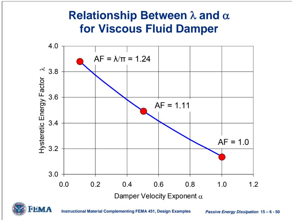
As indicated by the hysteretic energy factor, for a given force and displacement amplitude, the energy dissipated per cycle for a nonlinear fluid damper is larger than for a linear fluid damper and increases as the velocity exponent decreases. The amplification factor (AF) represents the factor by which the energy dissipated per cycle is increased for the nonlinear damper as compared to the linear damper (i.e.,  $AF = \text{hysteretic energy factor divided by } \pi$ ).
