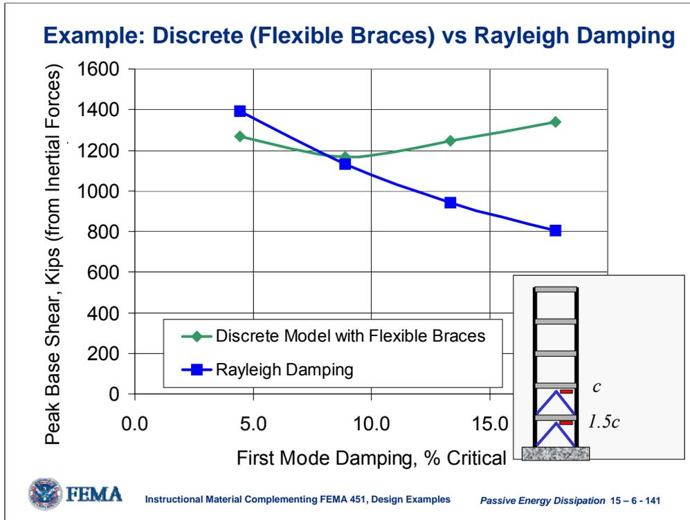
This slide is a continuation of the previous slide. There is significant deviation in the predicted peak base shear using the two damping matrices, particularly for higher levels of added damping.
