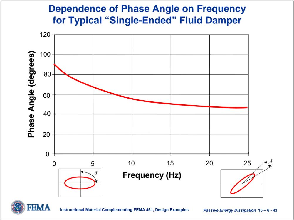
The phase angle between the peak displacement and peak force approaches 90 degrees as the frequency approaches zero. In this case, the storage stiffness is zero and the damper behaves as a pure viscous dashpot. As the frequency of motion increases, the phase angle reduces and the storage stiffness has a non-zero value.
