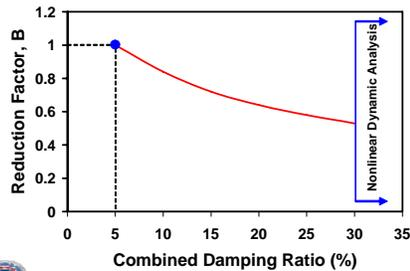
**Note:** After publication, it was recognized that this procedure may not be appropriate since it allows reduction in forces due to both inelastic structural response (R-factor) and added damping (B-factor). For yielding structures, added damping will not reduce forces.
