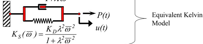
$$K_S(\bar{\omega}) = \frac{K_D \lambda^2 \bar{\omega}^2}{1 + \lambda^2 \bar{\omega}^2}$$
