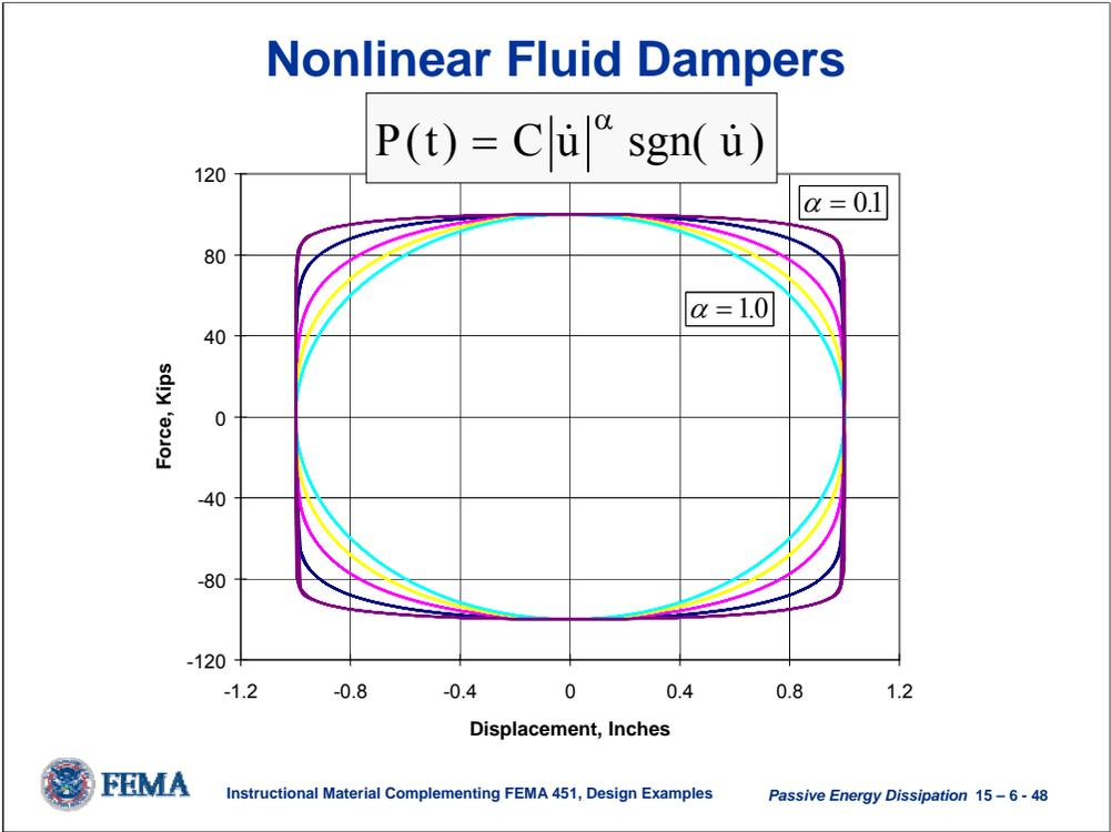
The hysteresis loops for nonlinear fluid dampers move from an ellipse for the linear case (velocity exponent = 1.0) to a rectangle (velocity exponent = 0.0). Thus, for a given force and displacement amplitude, the energy dissipated per cycle for a nonlinear fluid damper is larger than for a linear fluid damper.
