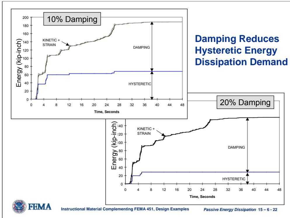
Energy response histories are shown for a SDOF elasto-plastic system subjected to seismic loading. An increase in added damping reduces the hysteretic energy dissipation demand by about 57%. Note that the input energy also changes since the input energy is dependent on the deformations of the structure. In this case, the input energy has reduced, although this is not always the case.
