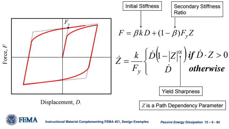
The hysteretic behavior of the ADAS device can be represented by various mathematical models. For example, SAP2000 and ETABS provides the analytical model shown here which was developed by Wen. This model can not capture the increasing stiffness at larger displacements.
