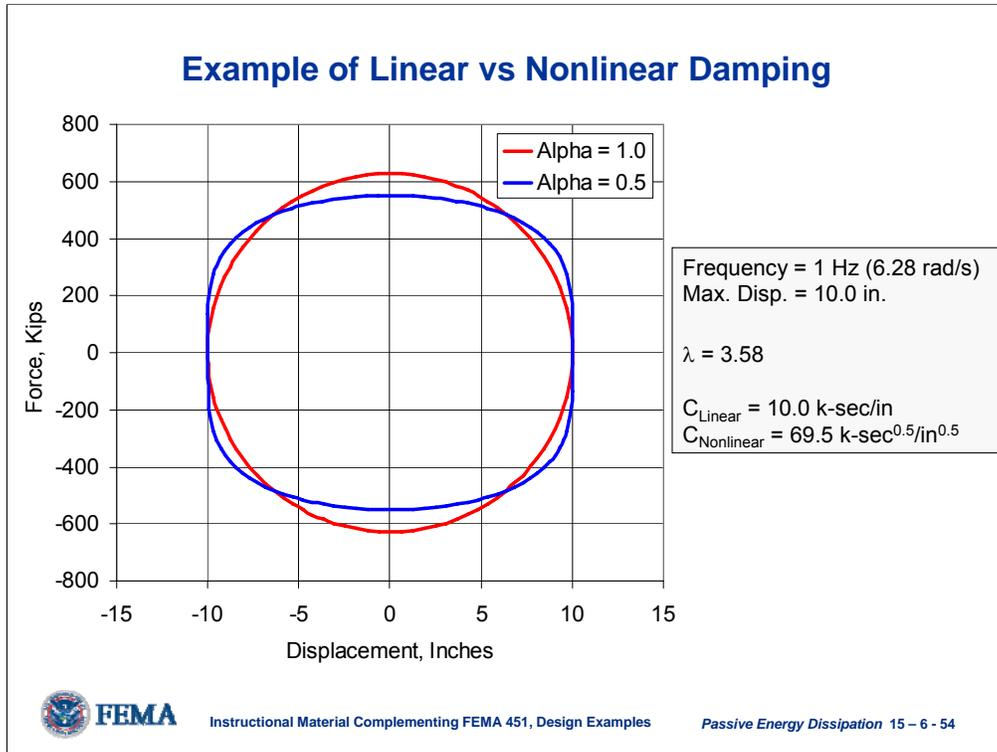
In this example, the  $C$  value for the nonlinear damper must be 6.95 times as large as for the linear damper to produce the same amount of energy dissipation per cycle for the identical harmonic loading conditions (i.e., same frequency and amplitude).
