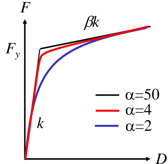
Degrading Stiffness, Degrading Strength, and Pinching Models also available. See Sivaselvan and Reinhorn for Details.
