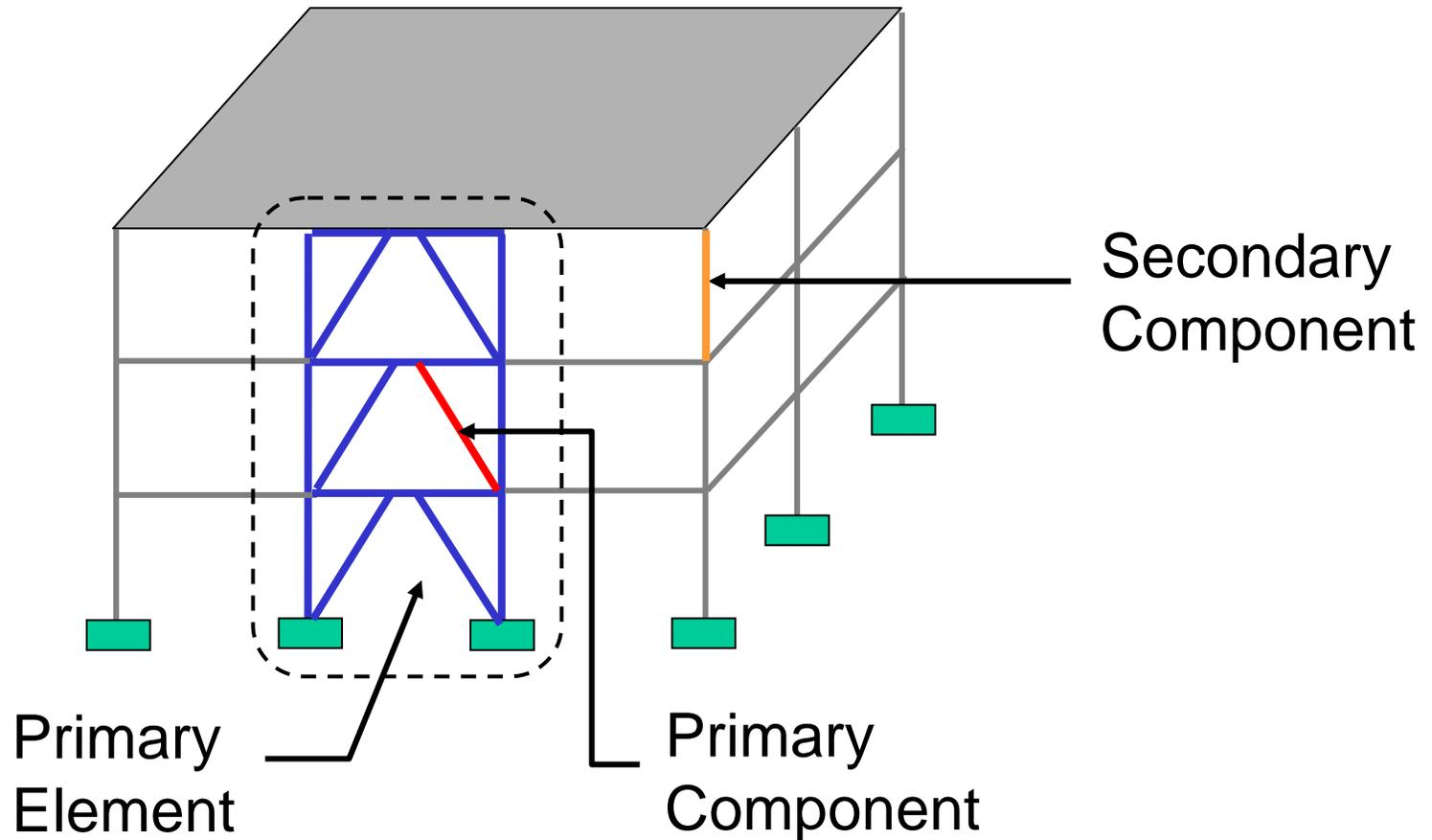
**Primary elements or components are critical to the buildings ability to resist collapse**
