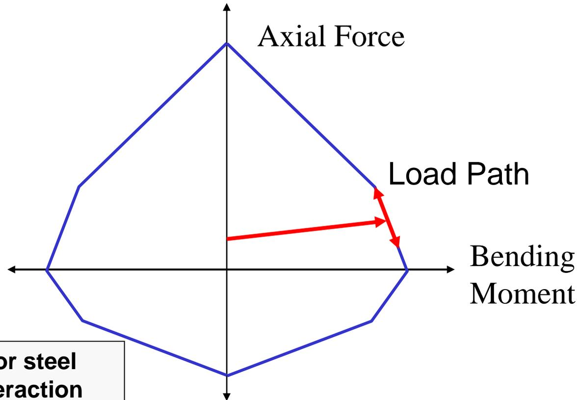
**Note: Diagram is for steel sections. NOo interaction and reinforced concrete type interaction is also possible**
