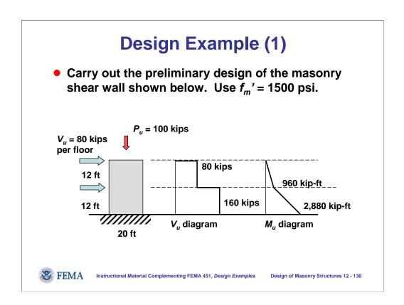
Now let's use those principles to carry out the preliminary design of a masonry shear wall. It measures 20 ft in plan; has two stories; and has factored lateral loads of 80 kips on each floor. Factored axial load is 100 kips. Factored design shear and moment diagrams are shown to the right of the slide.
