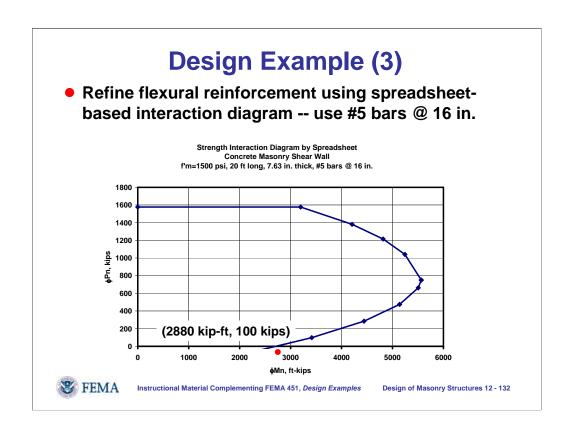
Using a spreadsheet-based program, calculate the interaction diagram for different assumed steel areas. The diagram shown is for #5 bars @ 16 in. The combination of factored actions (2880 kip-ft, 100 kips) lies within the diagram of design capacities.
