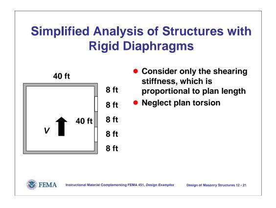
This process can be simplified considerably by neglecting plan torsion. This assumption is generally valid if the building has several walls oriented in each plan direction and well-distributed about the plan perimeter. It is not valid for garage-type buildings with one side almost completely open.
