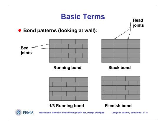
Masonry units can be laid in different bond patterns. The most common of these is 1/2 running bond, often called simply "running bond." Horizontal bed joints are continuous; vertical head joints alternate courses, and the head joint of one course aligns with the middle of the unit on the adjacent courses. In stack bond (referred to in the MSJC Code and Specification as "other than running bond"), the head joints are continuous between adjacent courses.
