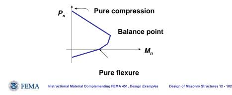
Using the assumptions of Section 3.3.2 of the MSJC Code, capacity of reinforced masonry elements under combinations of flexure and axial load is described using a moment-axial force interaction diagram, just as for reinforced concrete.
