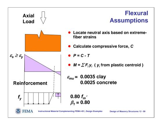
This slide summarizes how those flexural assumptions are applied. As will be discussed subsequently, sections are required to be tension-controlled so the strain gradient varies across the depth of the cross-section from the maximum useful strain in the masonry to a steel strain at least equal to yield. Reinforcement is considered to be elastoplastic. The equivalent rectangular stress block is taken as shown.
