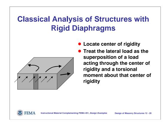
In a structure with a rigid diaphragm, the classic approach is first to locate the "center of rigidity," or shear center of the plan. The shear center is the point through which lateral forces must be applied so that the building will not twist in plan.
