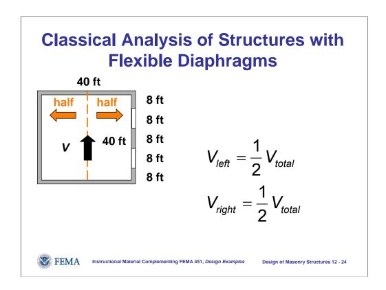
For the same building studied above but with a flexible diaphragm, the left and right shear walls each resist 1/2 the total lateral load.
