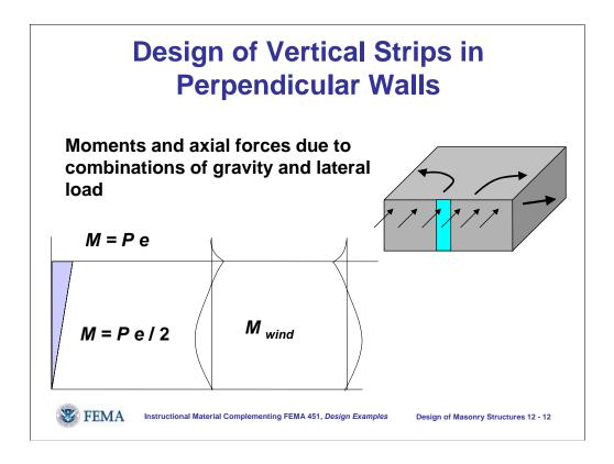
Vertically spanning strips in walls perpendicular to the direction of lateral load are subjected to axial load and possibly to eccentric gravity load from the roof.
