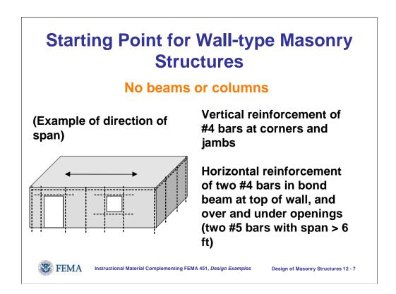
The starting point for low-rise, wall-type masonry structures is shown in this slide.
