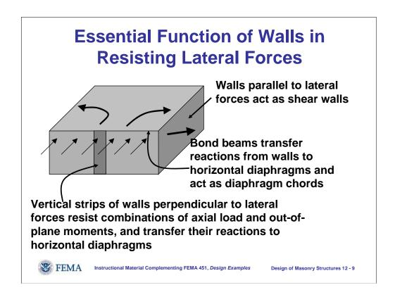
This slide shows how wall-type structures resist lateral loads.
