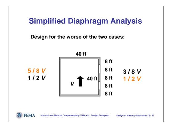
Further, it is possible to avoid the need to classify the diaphragm as "rigid" or "flexible." Simply design each wall for the more critical of the simplified rigid-diaphragm case and the flexible-diaphragm case.
