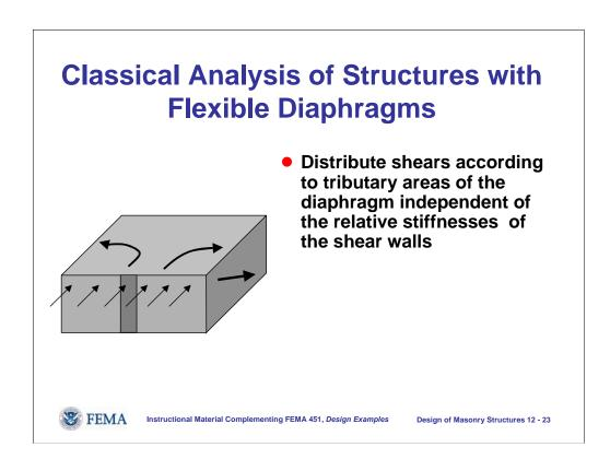
For buildings with flexible diaphragms, the diaphragm is idealized as a simply supported beam acting in the horizontal plane and resting on the shear walls. Because the shear walls are very stiff compared to the diaphragm, the shears on the shear walls depend on the tributary areas of the diaphragm that each shear wall supports.
