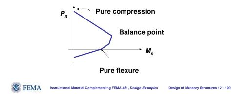
Walls are designed under out-of-plane loads using a strength interaction diagram.
