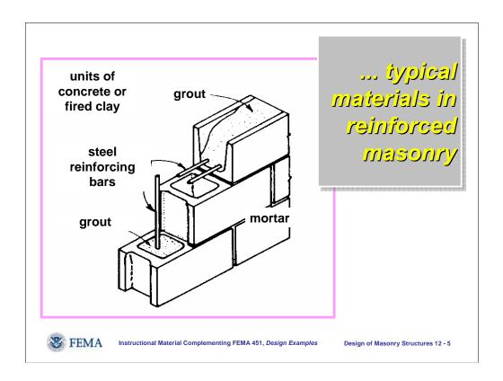
Modern reinforced masonry is commonly composed of hollow concrete or clay masonry units, jointed together by cementitious mortar. Deformed reinforcement is placed vertically and horizontally within voids in the masonry, which are then filled with grout, a fluid concrete-like mixture.
