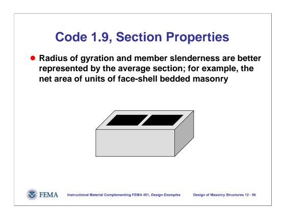
For computing slenderness-related properties, use the average section (the net area of units of face-shell bedded masonry).
