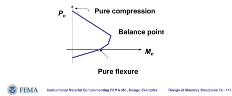
Flexural design of walls for in-plane loads is again handled using a strength interaction diagram. Because such walls have multiple layers of reinforcement over their depth, hand computations are tedious, and hand approximations (see design example at the end of this module) or computer spreadsheet calculations are preferable.
