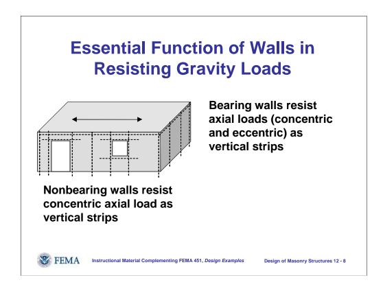
This slide shows how a wall-type building resists gravity loads. Nonbearing walls resist concentric axial loads from their own weight only. Bearing walls resist concentric axial loads from their own weight, and possibly eccentric axial loads from the reactions of roof elements. Both types of wall can be idealized as vertically spanning strips simply supported at the level of floor slab and horizontal diaphragms.
