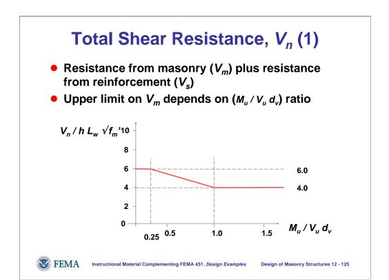
As discussed previously, total shear resistance is limited to prevent diagonal crushing of masonry.
