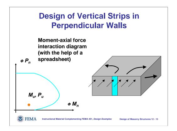
Design of the vertical strips consists simply of comparing the combination of factored design moment and axial load, with the design capacity expressed in terms of a moment-axial force interaction diagram, including the effects of  $\Phi$  factors.
