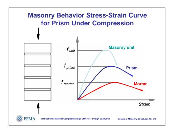
Compressive stress-strain behavior is evaluated using a masonry "prism" composed of units bonded by mortar and filled with grout (if it is intended to represent grouted construction). The individual behavior of units, mortar, and grout is not nearly as important as the behavior of the composite.
