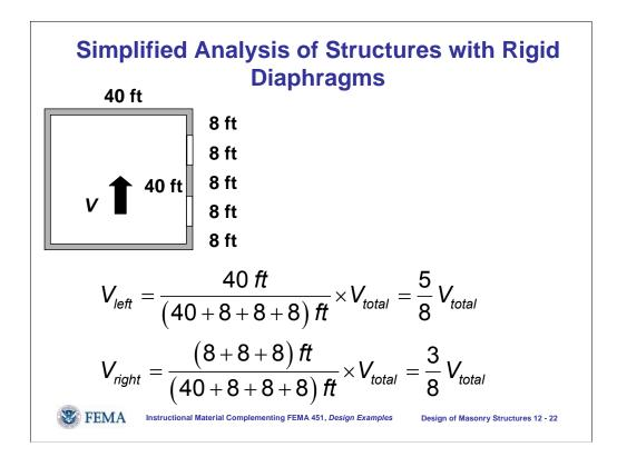
Consider the building plan shown above in which the wall on the left has a plan length of 40 ft and the wall on the right is composed of three segments with a plan length of 8 ft each.
