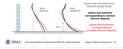
In checking shear capacity, the first step is to estimate the design shear.
