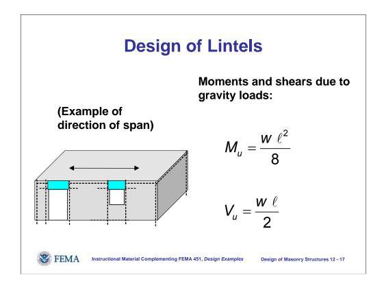
Lintels are beams that define openings in a wall.
