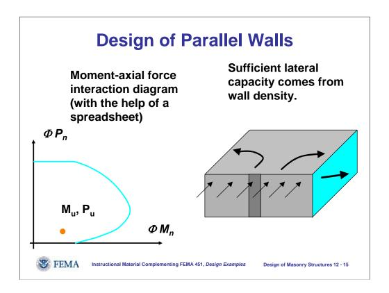
Flexural design of shear walls is expressed in terms of the relationship between combinations of factored moment and axial force and a momentaxial force interaction diagram.
