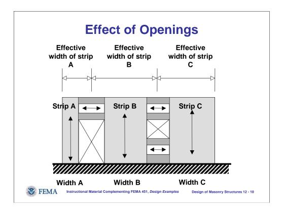
When walls oriented perpendicular to the direction of lateral load have door or window openings, these interrupt the path of vertical force transmission and change the design concept to a combination of horizontally spanning and vertically spanning strips.
