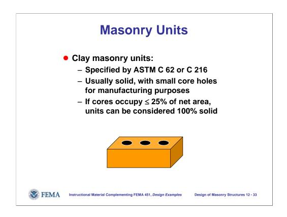
Clay masonry units are specified by ASTM C62 (building brick) or C216 (facing brick). They are usually solid and may have small core holes to facilitate drying and firing. Because clay masonry units usually have more than enough compressive strength, the core holes are ignored unless they occupy more than 25% of the area of the units.
