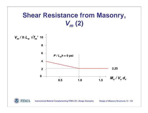
Shear resistance from masonry varies with aspect ratio as shown in this graph.
