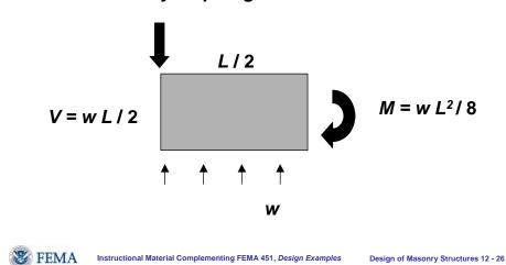
If the diaphragm is continuous, diaphragm shears are resisted by the total depth of the diaphragm. If the diaphragm is discontinuous, diaphragms are resisted by cover only. Flexural resistance comes from forces in diaphragm chords separated by the internal lever arm (distance between chords)
