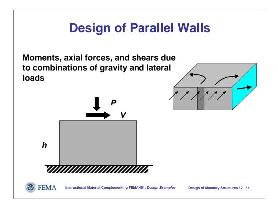
Parallel walls must be designed to resist shears from the diaphragms plus moments and axial forces.
