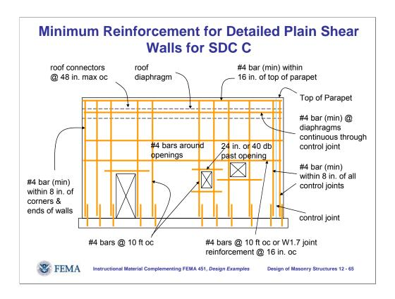
This slide illustrates the minimum reinforcement requirements for detailed plain masonry shear walls and for all shear walls in SDC C.
