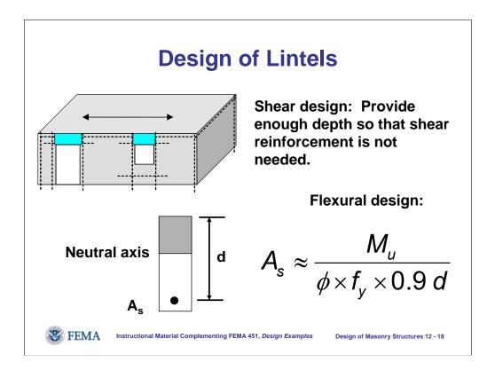
Design of the lintel for shear is quite simple. Because shear reinforcement is impractical for masonry lintels, the designer simply checks that the architecturally defined depth and width of the lintel give sufficient cross-sectional area so that shear reinforcement is unnecessary. Lintels should be grouted solid.
