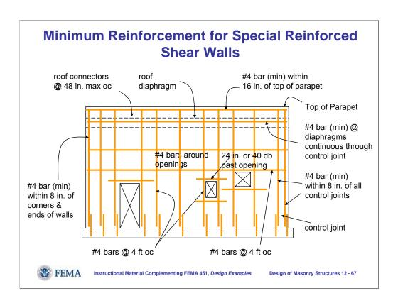
This slide illustrates the minimum reinforcement requirements for special reinforced masonry shear walls.
