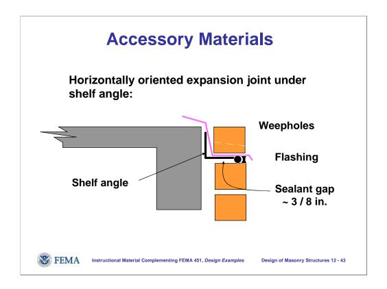
One of the most important details in a masonry building is the expansion joint under shelf angles in clay masonry veneer. Clay masonry expands over time; concrete and concrete masonry shrink. If the veneer is laid without the expansion joint, it will end up supporting the building even though it is not made to resist the resulting compression.
