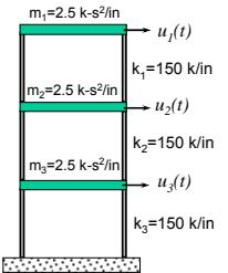
$$\begin{aligned} \ddot{y}_1 + 2\xi_1\omega_1\dot{y}_1 + \omega_1^2 y_1 &= V_1^*(t)/m_1^* \\ \ddot{y}_2 + 2\xi_2\omega_2\dot{y}_2 + \omega_2^2 y_2 &= V_2^*(t)/m_2^* \\ \ddot{y}_3 + 2\xi_3\omega_3\dot{y}_3 + \omega_3^2 y_3 &= V_3^*(t)/m_3^* \\ \ddot{y}_1 + 0.345\dot{y}_1 + 11.88y_1 &= -1.22\ddot{v}_g(t) \\ \ddot{y}_2 + 0.966\dot{y}_2 + 93.29y_2 &= 0.280\ddot{v}_g(t) \\ \ddot{y}_3 + 1.395\dot{y}_3 + 194.83y_3 &= -0.06\ddot{v}_g(t) \end{aligned}$$
