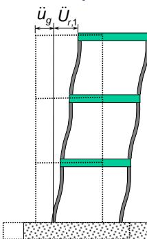
$$F_j(t) = M \begin{Bmatrix} \ddot{u}_g(t) + \ddot{u}_{r,1}(t) \\ \ddot{u}_g(t) + \ddot{u}_{r,2}(t) \\ \ddot{u}_g(t) + \ddot{u}_{r,3}(t) \end{Bmatrix} =$$
