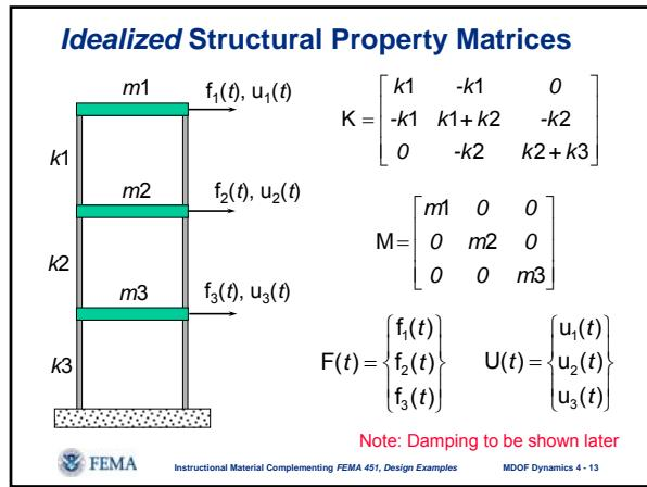
**Coupled Equations of Motion for Undamped Forced Vibration**
