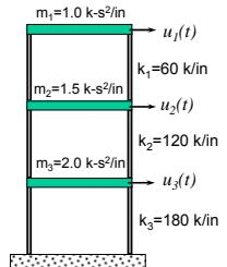
$$\begin{aligned}\ddot{y}_1 + 2\xi_1\omega_1\dot{y}_1 + \omega_1^2 y_1 &= V_1^*(t) / m_1^* \\ \ddot{y}_2 + 2\xi_2\omega_2\dot{y}_2 + \omega_2^2 y_2 &= V_2^*(t) / m_2^* \\ \ddot{y}_3 + 2\xi_3\omega_3\dot{y}_3 + \omega_3^2 y_3 &= V_3^*(t) / m_3^*\end{aligned}$$
