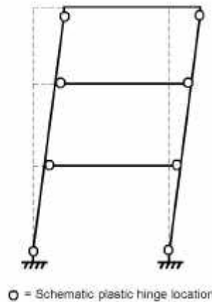
Figure C6.15.4.3.1.e-1: Acceptable plastic mechanism for multi-tier bent.
