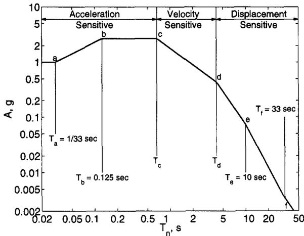
Figure 2. Newmark-Hall elastic design spectrum.
