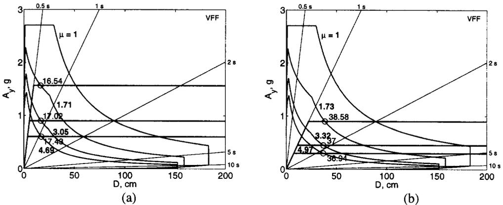
Figure 11. Application of improved Procedure A using Vidic-Fajfar-Fischinger (1994) inelastic design spectrum: (a) Systems 1 to 3, and (b) Systems 4 to 6.
