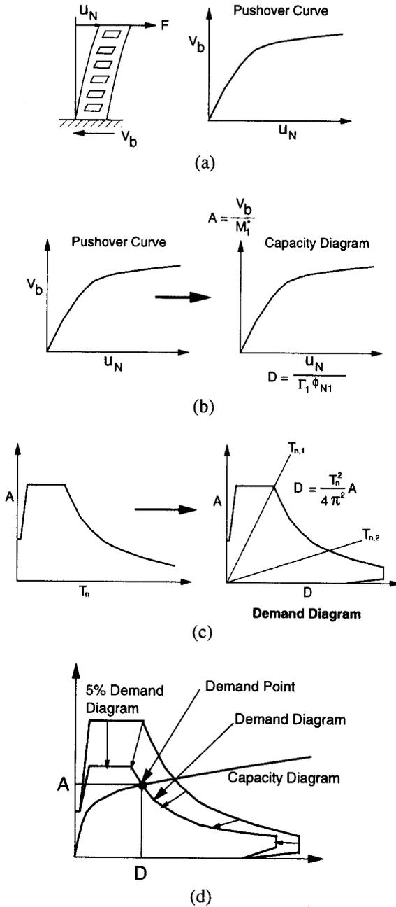
**Figure 1.** Capacity spectrum method: (a) development of pushover curve, (b) conversion of pushover curve to capacity diagram, (c) conversion of elastic response spectrum from standard format to A-D format, and (d) determination of displacement demand.
