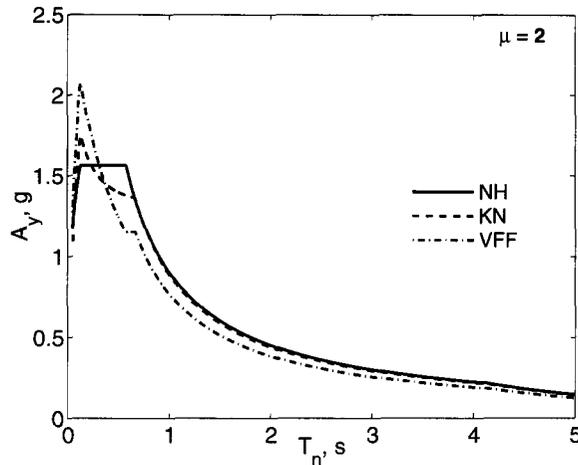
**Figure 7.** Pseudo-acceleration design spectrum for inelastic systems ( $\mu=2$ ) using three  $R_y - \mu - T_n$  equations: Newmark-Hall (NH), Krawinkler-Nassar (KN), and Vidic-Fajfar-Fischinger (VFF).
