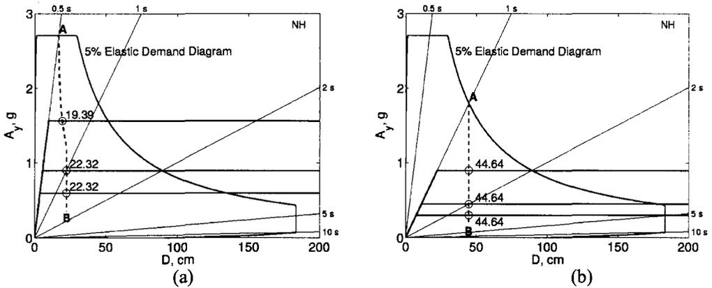
Figure 12. Application of improved Procedure B using Newmark-Hall (1982) inelastic design spectrum: (a) Systems 1 to 3, and (b) Systems 4 to 6.
