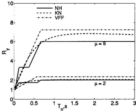
**Figure 13.** Variation of  $R_y$  with  $T_n$  for selected ductility values based on three different sources: Newmark and Hall (1982), Krawinkler and Nassar (1992), and Vidic, Fajfar, and Fischinger (1994).
