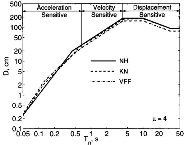
**Figure 3.** Deformation of inelastic systems ( $\mu = 4$ ) determined from inelastic design spectra using three  $R_y - \mu - T_n$  equations: Newmark-Hall (NH), Krawinkler-Nassar (KN), and Vidic-Fajfar-Fischinger (VFF).
