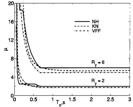
**Figure 14.** Variation of  $\mu$  with  $T_n$  for selected  $R_y$  values based on three different sources: Newmark and Hall (1982), Krawinkler and Nassar (1992), and Vidic, Fajfar, and Fischinger (1994).
