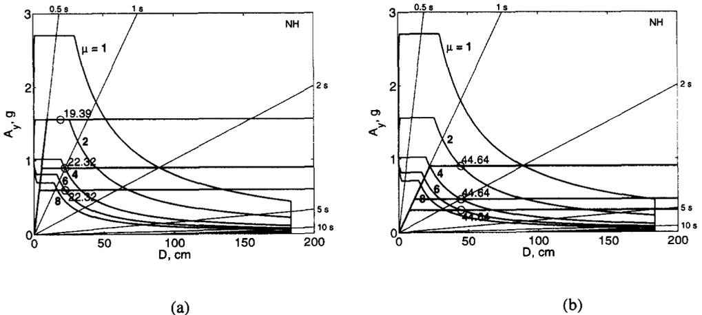
**Figure 9.** Application of improved Procedure A using Newmark-Hall (1982) inelastic design spectrum: (a) Systems 1 to 3, and (b) Systems 4 to 6.
