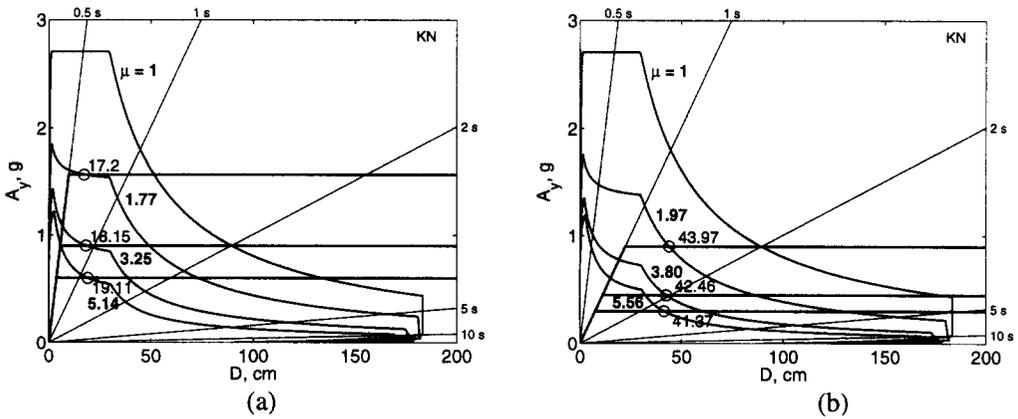
Figure 10. Application of improved Procedure A using Krawinkler-Nassar (1992) inelastic design spectrum: (a) Systems 1 to 3, and (b) Systems 4 to 6.
