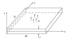
The plate surfaces are at  $z = \pm t/2$ , and its midsurface is at z = 0.
