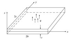
2. The deflection *w* is much less than the thickness *t* (than is, *w/t* << 1).
