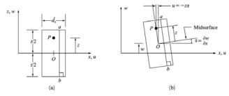
Loading q causes the plate to deform laterally or upward in the z direction and, the defection w of point P is assumed to be a function of x and y only; that is w = w(x, y) and the plate does not stretch in the z direction.
