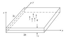
If *t* is more than about one-tenth the span of the plate, then transverse shear deformation must be accounted for and the plate is then said to be thick.
