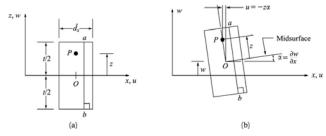
4. Therefore, the in-plane deflections in the x and y directions at the midsurface, z = 0, are assumed to be zero; u(x, y, 0) = 0 and v(x, y, 0) = 0.
