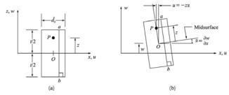
4. Membrane or in-plane forces are neglected here, and the plane stress resistance can be superimposed later (that is, the constant-strain triangle behavior of Chapter 6 can be superimposed with the basic plate bending element resistance).
