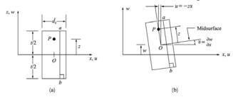
The line *a-b* drawn perpendicular to the plate surface before loading remains perpendicular to the surface after loading.
