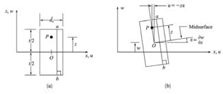
1. Normals remain normal. This implies that transverse shears strains  $\gamma_{yz} = 0$  and  $\gamma_{xz} = 0$ . However  $\gamma_{xy}$  does not equal to zero. Right angles in the plane of the plate may not remain right angles after loading. The plate may twist in the plane.
