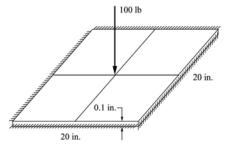
The exact solution for the displacement at the center of the plate is  $w = 0.0056PL^2/D$ .
