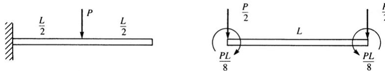
We will use one element and replace the concentrated load with the appropriate nodal forces.
