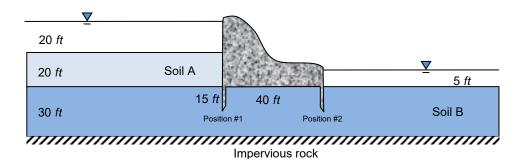
The upstream and downstream boundaries should be taken as impervious. This approximation is accurate if the boundaries are far from the dam. As part of your analysis, show the effect of moving these boundaries away from the dam. Demonstrate this on the Case I only.
