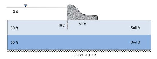
The upstream and downstream boundaries should be taken as impervious. This approximation is accurate if the boundaries are far from the dam. As part of your analysis, show the effect of moving these boundaries away from the dam. Demonstrate this on the Case I only.
