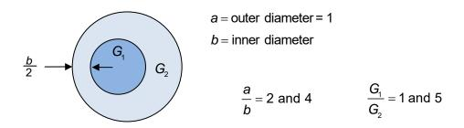
Use **POIS36** to the model this problem for the various cases indicated by the ratios a/b and  $G_1/G_2$ . From these results plot the stress function and calculate the torque on the cross-section. See - J.F. Ely and O.C. Zienkiewicz, "Torsion of compound bars - a relaxation solution." Int. J. Mech. Sci. Vol 1, pp. 356-365, 1960.
