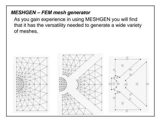
When it cannot be made to produce exactly a desired configuration (for example, nodal points on the boundary of loop 1 not lying in a prefect circle), the user may use MESHGEN to obtain a mesh very close to that which is desired, and then manually adjust whatever data are necessary to achieve the geometry required.
