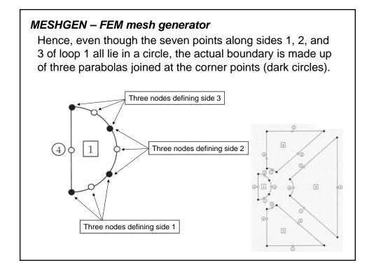
Although three of the 4 sides of loops 2, 3, and 4 are straight lines, the side coordinate points (open circles) do not necessarily fall at the center of these sides.
