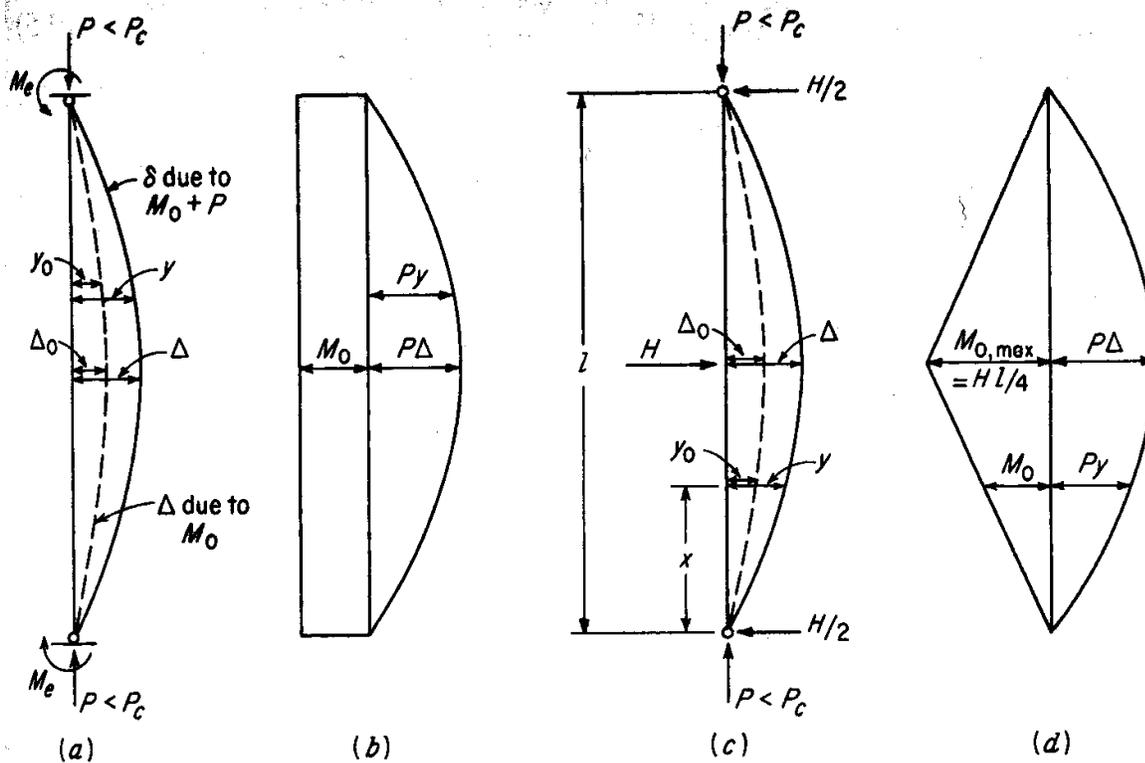
Figure 4. Moments in Slender Members with Compression plus Bending, Bent in Single Curvature.
