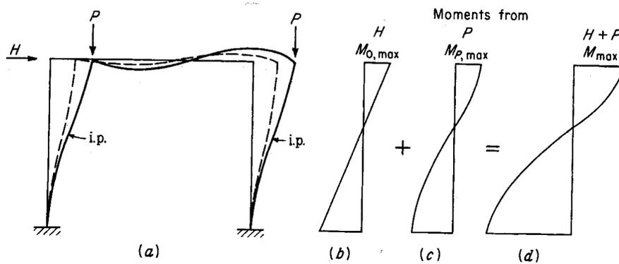
Figure 7. Fixed Portal Frame, Laterally Unbraced.
