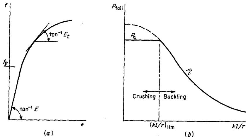
Figure 1. Effect of Slenderness on Strength of Axially Load Column.
