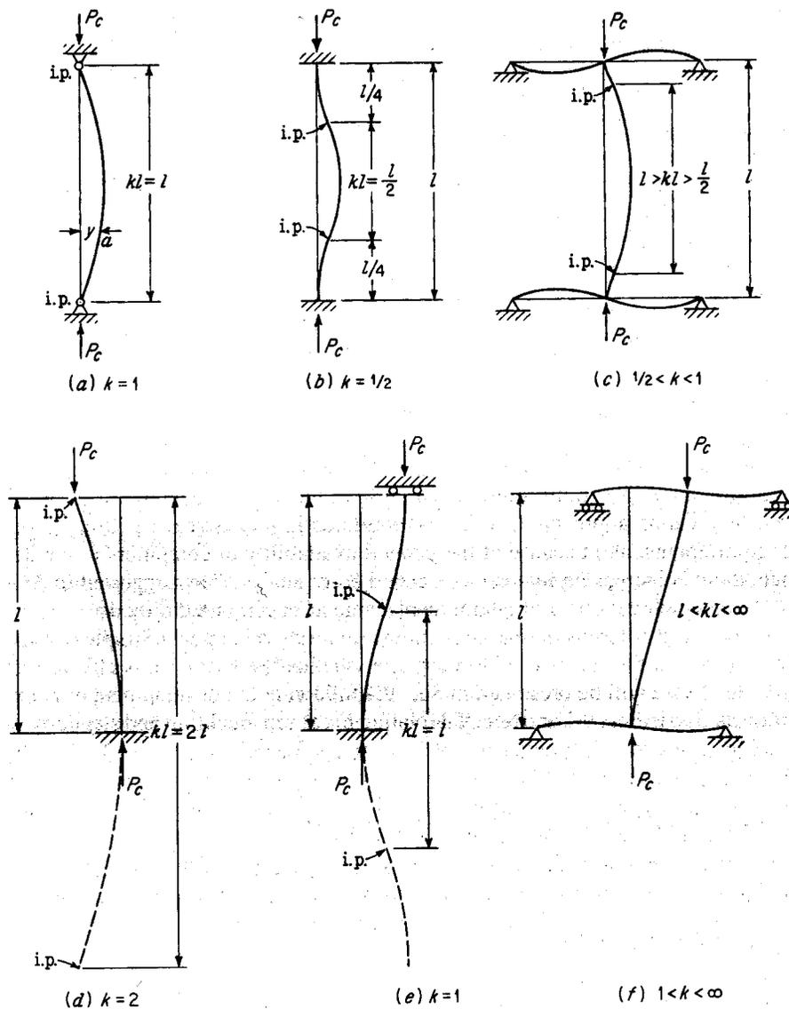
Figure 2. Buckling and Effective Length of Axially Loaded Columns.
