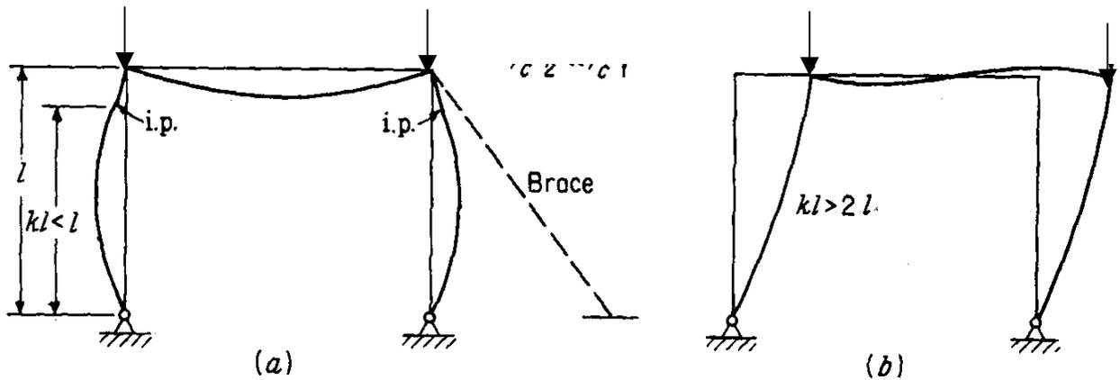
Figure 3. Rigid Frame Buckling: (a) Laterally Braced; (b) unbraced.
