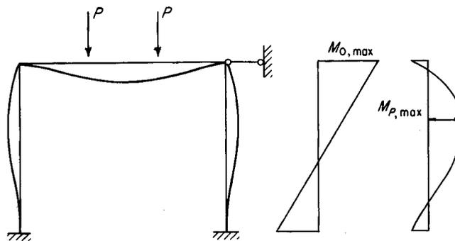
Figure 8. Fixed Portal Frame, Laterally Braced.
