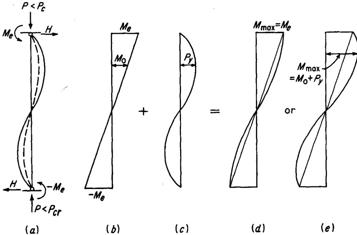
Figure 6. Moments in Slender Members with Compression Plus Bending, Bent in Double Curvature.
