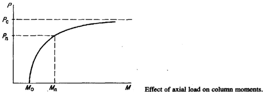
Figure 5. Effect of slenderness and Effect of Axial Load on Column Moments.
