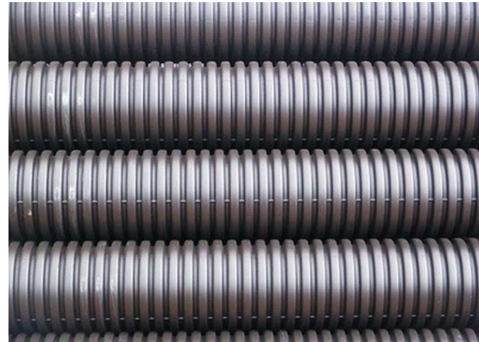
Corrugated Drain Pipe n = 0.024
