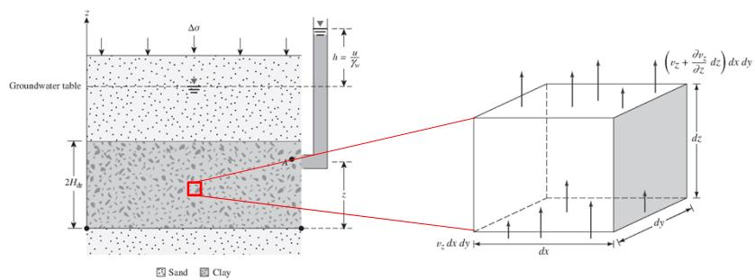
$$\frac{k}{\gamma_w} \frac{\partial^2 u}{\partial z^2} = \frac{a_v}{1 + e_o} \frac{\partial u}{\partial t} \quad \longrightarrow \quad \frac{\partial u}{\partial t} = c_v \frac{\partial^2 u}{\partial z^2}$$
