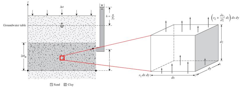
$$\frac{\partial v_z}{\partial z} dx dy dz = \frac{\partial V}{\partial t} \quad \longrightarrow \quad -\frac{k}{\gamma_w} \frac{\partial^2 u}{\partial z^2} = \frac{1}{1+e_o} \frac{\partial e}{\partial t}$$
