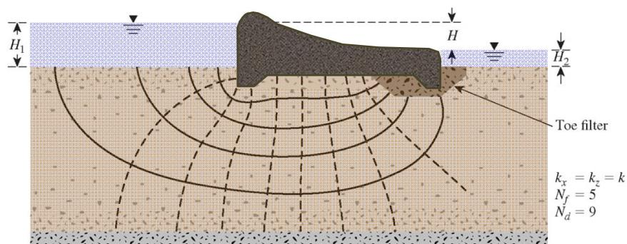
Flow lines are  $\perp$  to upstream ground surface
