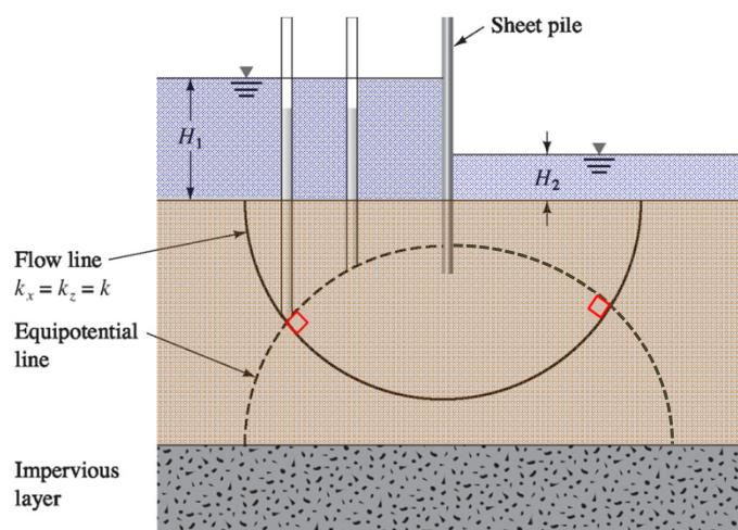
Flow lines and equipotential lines are orthogonal
