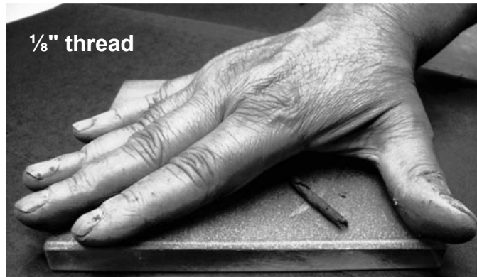
Figure 3.14 Plastic limit test (Courtesy of Braja M. Das, Henderson, Nevada)
