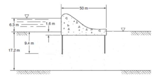
$$q = kH \frac{N_f}{N_d} = (8.4 \times 10^{-6} \ m/s)(6.3 \ m) \frac{3}{12} = 13.23 \times 10^{-6} \ m^2/s = 1.14 \ m^2/day \ per \ meter \ of \ width$$
