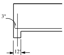
This is to ensure that the continued steel is of sufficiently small diameter and the required anchorage requirement of the ACI code is satisfied.
