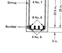
Final moment capacity with the chosen dimensions and reinforcing stee
