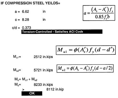
IF COMPRESSION STEEL DOES NOT YEILD=  $C_s = A'_s f'_s = A'_s \varepsilon'_s E_s = A'_s \left( 0.003 \frac{c-d}{c} \right)$  $E_s$  $\overline{C_c} = 0.85 f_c' \beta_1 cb$  $T_{s} = A_{s}f_{v}$ Equilibrium = kips C = 7.33 in -45 Moment Force Arm Cs = 136 19.70 2677 Cc = 19.27 5762 299 Ts= 480 0.00 0 in-kips Mn = 8439 Mu = 7567 in-kips 8112 in.kip ngth Requiremen Mn =703 ft-kips 631 ft-kips Mu =
