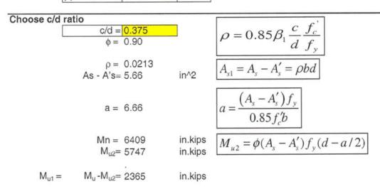
Find the compression steel. First check to see if the compression steel will yield at failure
