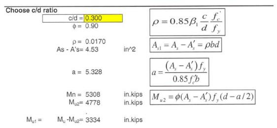
Find the compression steel. First check to see if the compression steel will yield at failure
