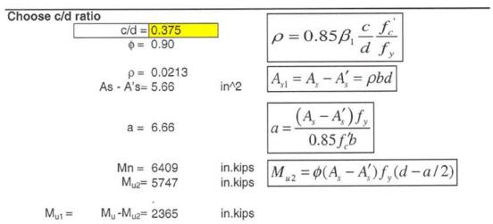
Find the compression steel. First check to see if the compression steel will yield at failure
