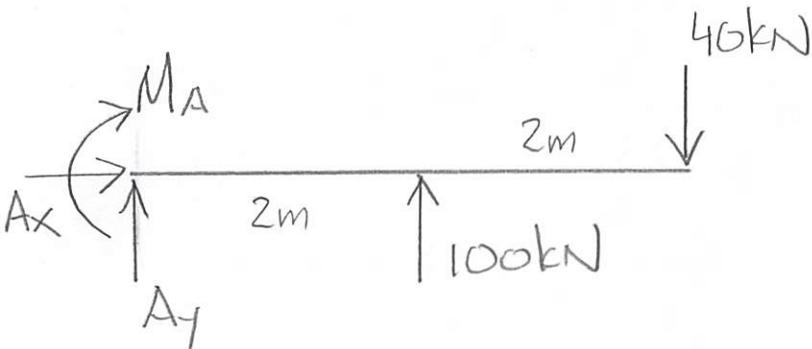
$$\begin{aligned} \sum M_A &= 0 \\ &= -M_A + 100\text{kN}(2\text{m}) - 40\text{kN}(4\text{m}) \end{aligned}$$
