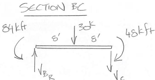
$$\begin{aligned} \text{At } B: \sum M_B &= 0 = 84\text{kft} - 48\text{kft} - 30\text{k}(8') - V_c(16') \\ V_c &= -12.75\text{k} \\ + \uparrow \sum F_y &= 0 = V_{B_R} - V_c - 30\text{k} \\ V_{B_R} &= +7.25\text{k} \end{aligned}$$
