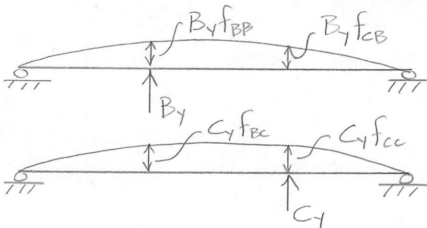
Problem 11-6 – Determine the support reactions. The supports at A, B, C, and D are pins. Assume the horizontal reactions are zero. EI is constant.
