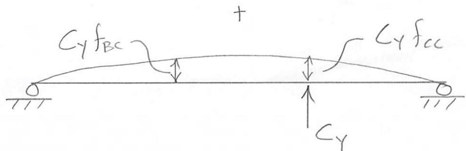
Problem 11-6 – Determine the support reactions. The supports at A, B, C, and D are pins. Assume the horizontal reactions are zero. EI is constant.
