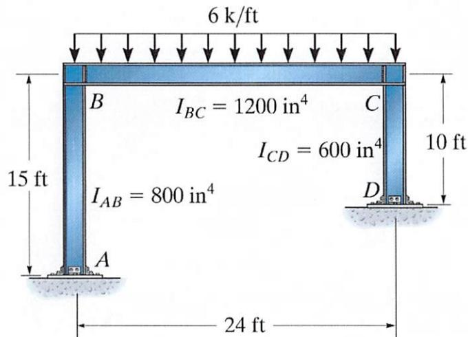
$$\underline{I_{AB} = \frac{4}{3} I_{CD}} \quad \underline{I_{BC} = 2 I_{CD}} \quad \psi = \frac{\Delta}{L}$$
