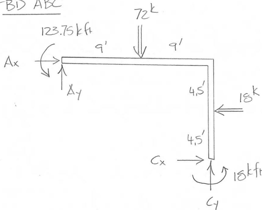
$$\begin{aligned} \textcircled{+} \sum M_C = 0 &= 18 \text{kft} + 123.75 \text{kft} + 72 \text{k}(9') \\ &\quad + 18 \text{k}(4.5') - A_y(18') - A_x(9') \end{aligned}$$
