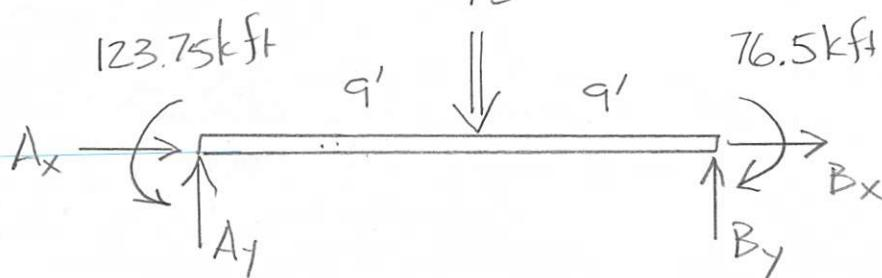
$$\begin{aligned} \textcircled{+} \sum M_B = 0 &= -76.5 \text{kft} + 123.75 \text{kft} + 72 \text{k}(9') \\ &\quad - A_y(18') \\ A_y &= \underline{38.63 \text{k}} \end{aligned}$$
