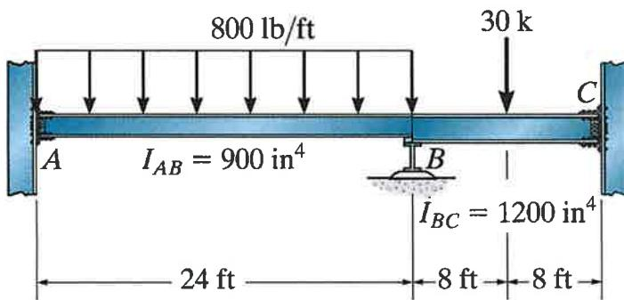
$$M_{BA} + M_{BC} = 0 = \frac{2E I_{AB}}{24 \text{ ft}} [2\theta_B] + 38.4 \text{ kft} + \frac{2E(\frac{4}{3} I_{AB})}{16 \text{ ft}} [2\theta_B] - 60 \text{ kft}$$
