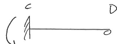
Problem 10a-3 – Determine the internal moments at the supports B and C. Assume  $EI$  is constant.
