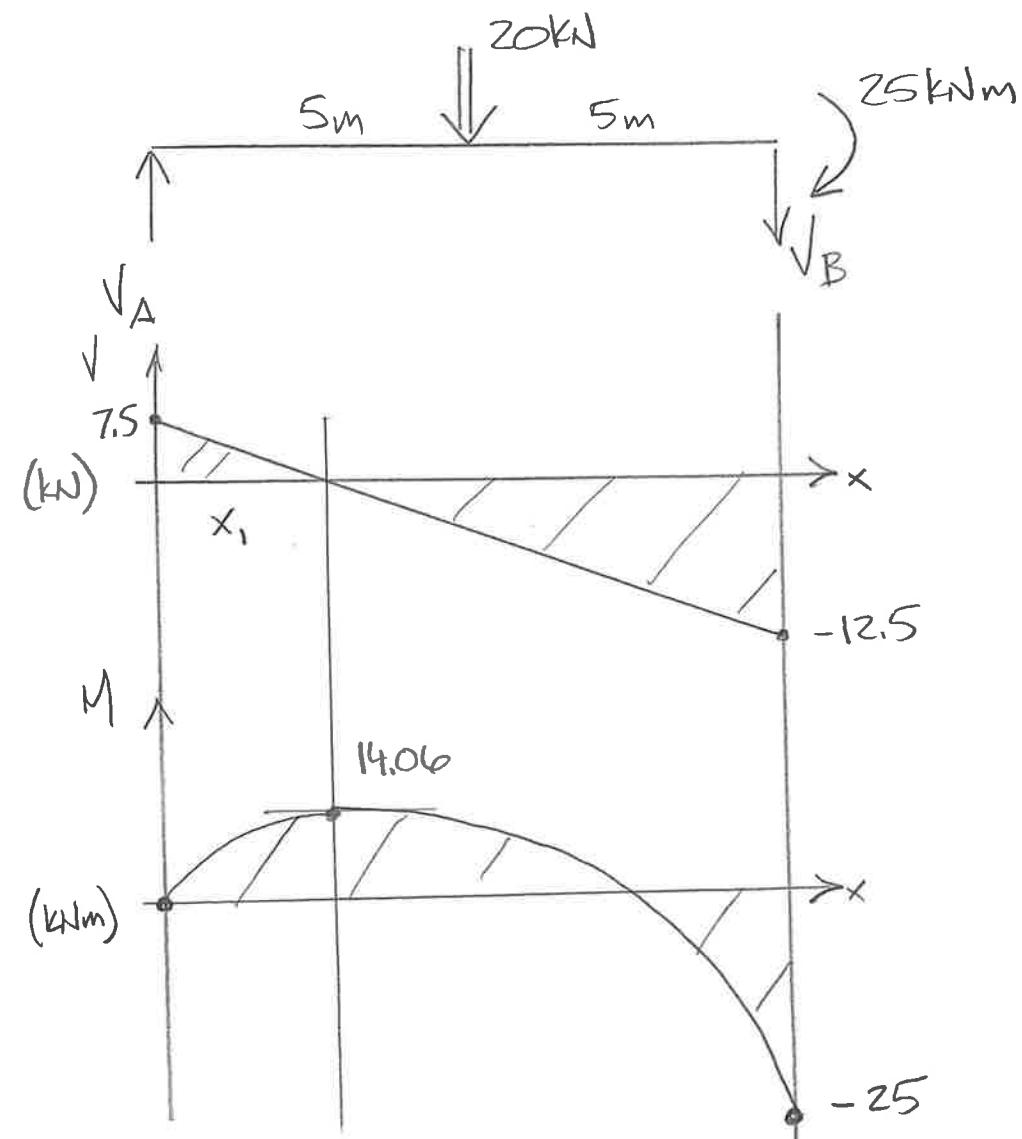
$$\begin{aligned} \text{At } A: \sum M_A &= 0 = -20\text{kN}(5\text{m}) - 25\text{kNm} \\ &\quad - V_B(10\text{m}) \end{aligned}$$
