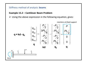
Stiffness method of analysis: beams
