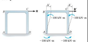
Displacement method of analysis: moment distribution for frames
