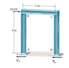
$\rightarrow^{+} \sum F_{x} = 0 = -V_{A} - V_{D} + 10 \, kN$
