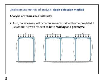
Displacement method of analysis: slope-defection method
